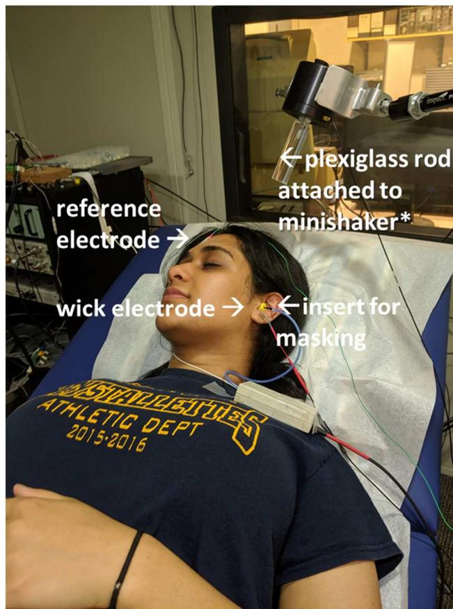
**Figure 2:** Mini-shaker and placement of electrodes. Please note ground electrode (M2; left mastoid process) is not shown in this image.
