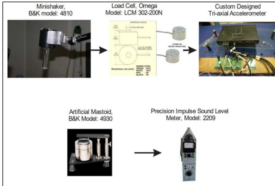
**Figure 3:** Signal path for calibration of the B&K mini-shaker
