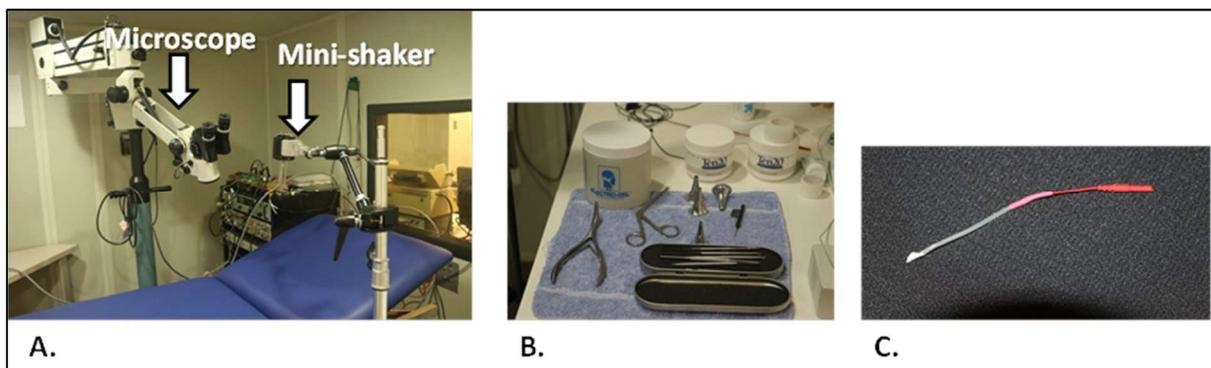
**Figure 1:** Special equipment for VsEPs A) operating microscope, examination table, and mini-shaker attached to an articulating stand B) tools to enhance TM visualization and placement (i.e., nasal speculum, electrode gel, etc) C) Lilly Wick electrode
