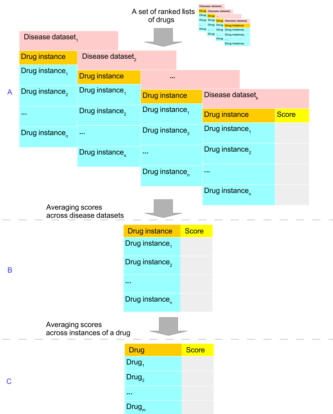
Figure 2: A systematic method [205] to select repurposing drug candidates. A) Given a set of ranked lists of drugs (drug instances), we compute a score for each drug. B) We then calculate an average score for each drug instance across different lists (using disease datasets). C) Finally, we calculate an average score for each distinct drug across the instances, in case there are multiple instances for that drug.
