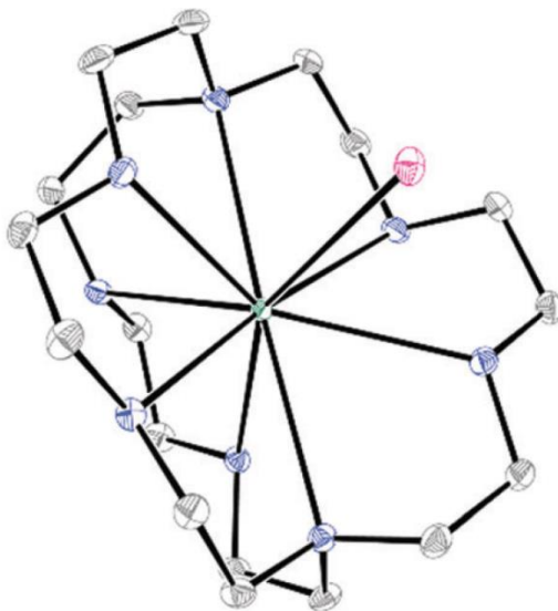
Figure 3.3 Crystal structure of \text{Eu23I}_2 . Hydrogen atoms and an outer-sphere iodide ion have been omitted for clarity. Thermal ellipsoids are drawn at 50% probability. Crystallographic data for this structure are available at the Cambridge Crystallographic Data Centre under deposition number CCDC 1826977. Blue = nitrogen; grey = carbon; seagreen = europium; and pink = iodine. Data collected by Philip D. Martin.
