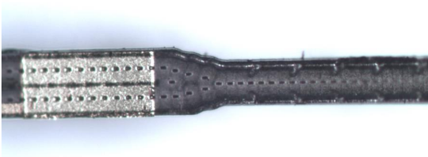
Figure 3-4. The distal end of the parylene tube.
