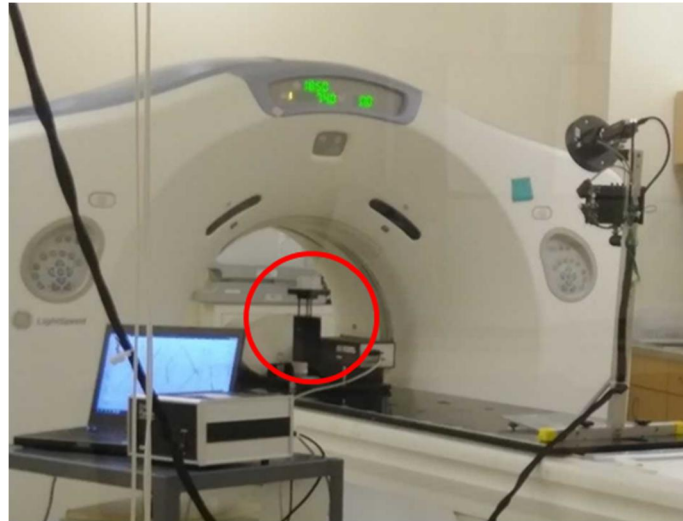
Figure 0-1: 4DCT of Lung Thoracic Motion Phantom using RPM
