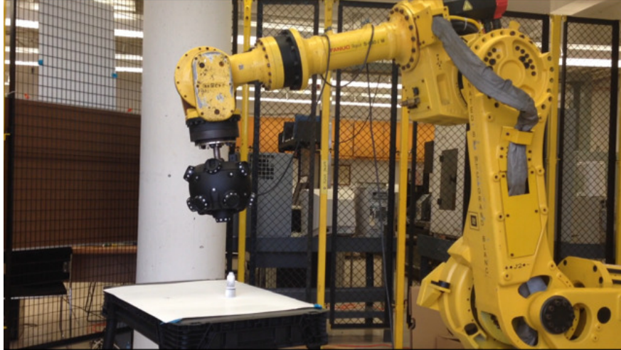
Figure 1.4: Triangulation scanners or shape scanners attached to a robot
