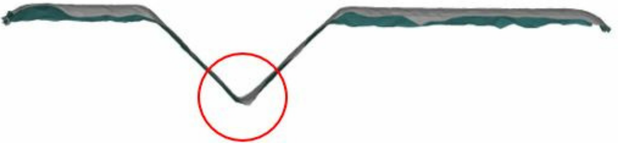
Figure 4.7: The shape of the scanned point cloud representing the defect after meshing the points.
