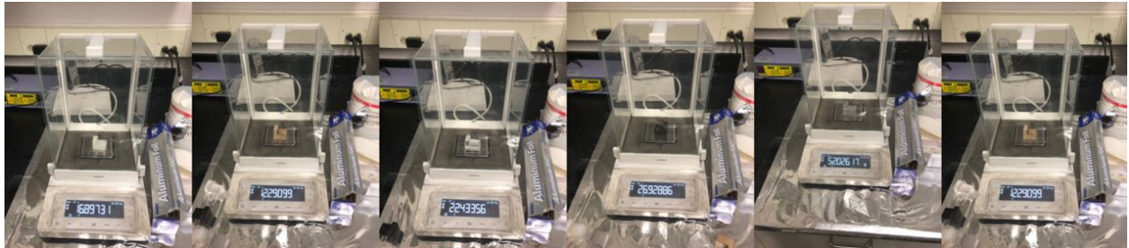
Figure 5.2: Selected materials weight on a high precision scale to calculate density
