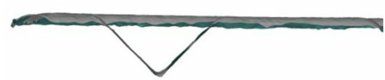
Figure 4.8: The shape of the scanned point cloud of a defective part aligned with the scanned point cloud of an intact part.
