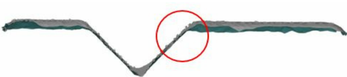
Figure 4.3: Effect of the slice height on the manufacturing error
