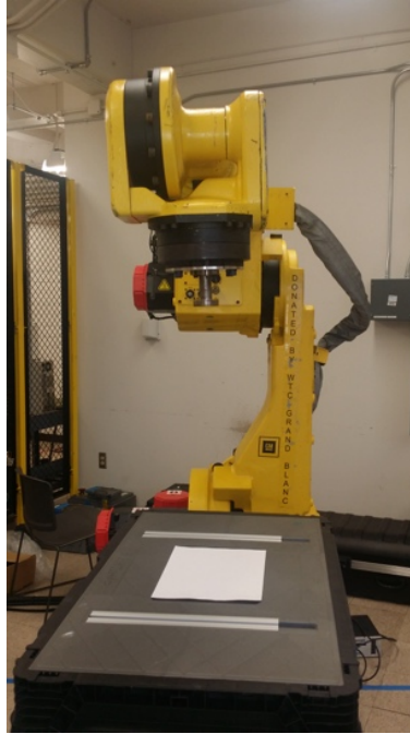
Figure 2.4: The robot calibrated and set up at zero position without the Scanner installed
