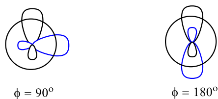
Figure 13. Interactions of non-bonding orbitals of nitrogen atoms at \phi = 90^\circ and 180^\circ .
