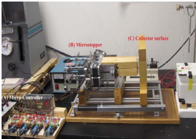
Figure 10 . Prototype of automatic NF collector device. (A) Micro-controller; (B) Microstepper, and (C) collector surface
