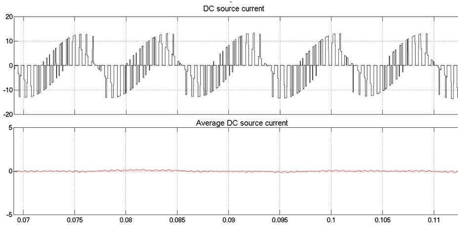
Fig. 49. DC source current of the SSBC circuit.
