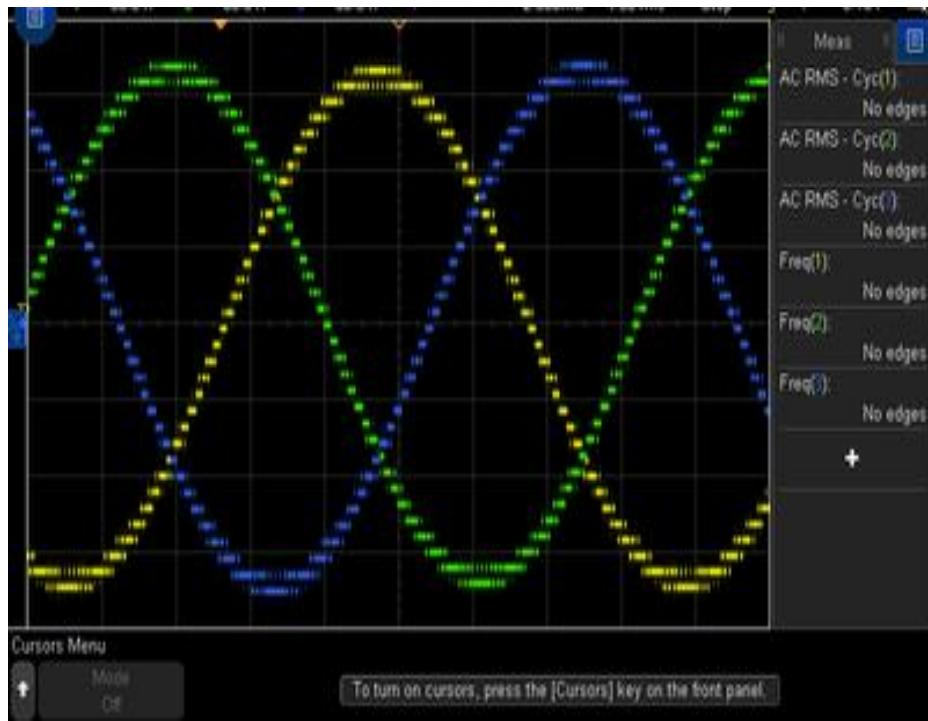
Fig. 42. Experimental voltage waveforms of 33-level HCMC inverter.
