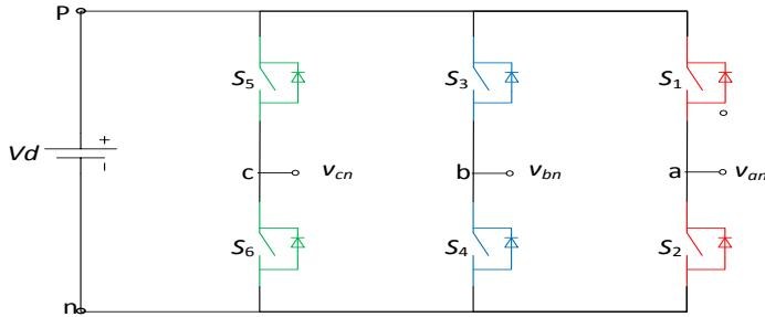
Fig. 11. Three-phase inverter.
