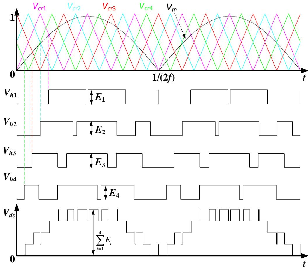
Fig. 29. Phase-shifted PWM modulation for a nine-level HCMC.
