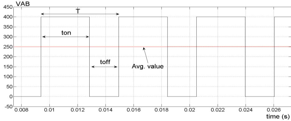
Fig. 8. Output waveform for half-bridge converter:  $V_d= 400V$  and  $d= 0.625$ .
