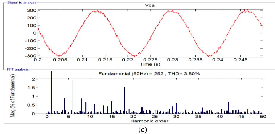
Fig. 48. SSBC connected to the HCMC system: (a), (b), (c) are L-L voltage waveforms with their THD ( $m_{i,a}=1$ ,  $m_{i,b}=0.9$ ,  $m_{i,c}=0.95$ , fundamental frequency= 60Hz, and carrier frequency= 360 Hz).
