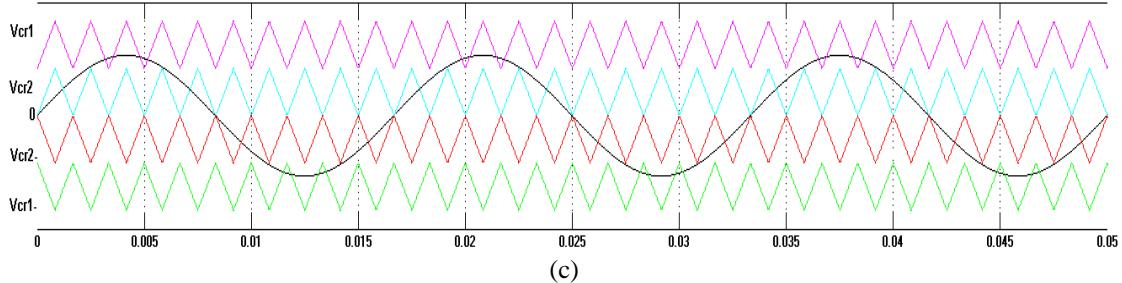
Fig. 19. Five-level converter: three techniques for level-shifted PWM scheme (a) In-phase disposition (IPD), (b) Alternative phase opposite disposition (APOS), and (c) Phase opposite disposition (POD).
