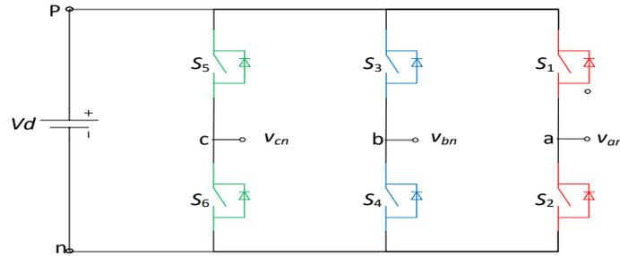
Fig. 11. Three-phase inverter.
