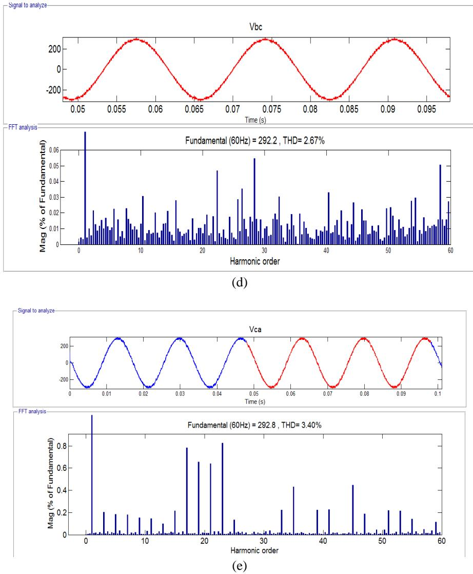
Fig. 37. Bypassing a battery module: (a) Current of bypassed cell ( $m_{i,x}=0$ ), (b) Current of other healthy battery cells ( $m_{i,x}>1$ ), (c), (d), (e) are the line to line output voltage waveforms with their THD values after bypassing a battery from phase A.
