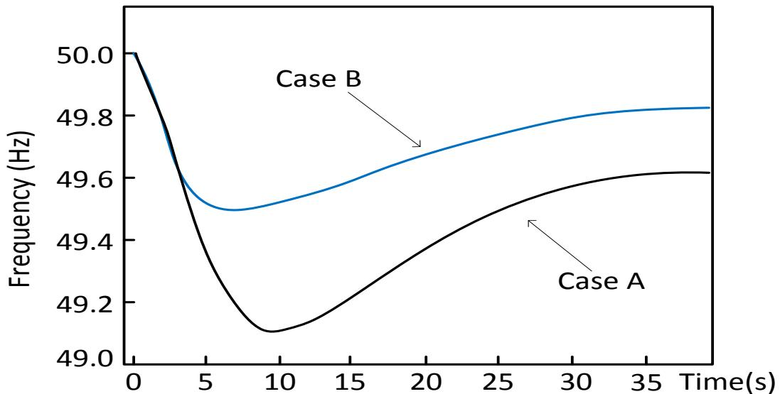
Fig. 1. Hydrothermal power system frequency response with/without BESS [12].
