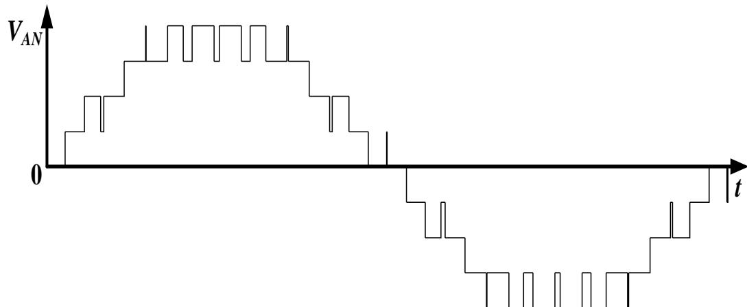
Fig. 30. Output voltage of nine-level HCMC multilevel inverter ( $m_i=0.95$ , fundamental frequency= 60Hz, and carrier frequency= 180 Hz).
