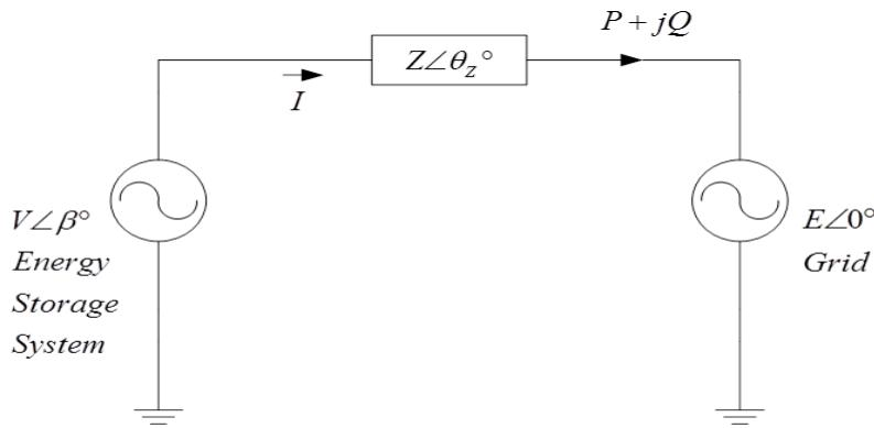
Fig. 33. Single diagram of BESS connected to utility grid.
