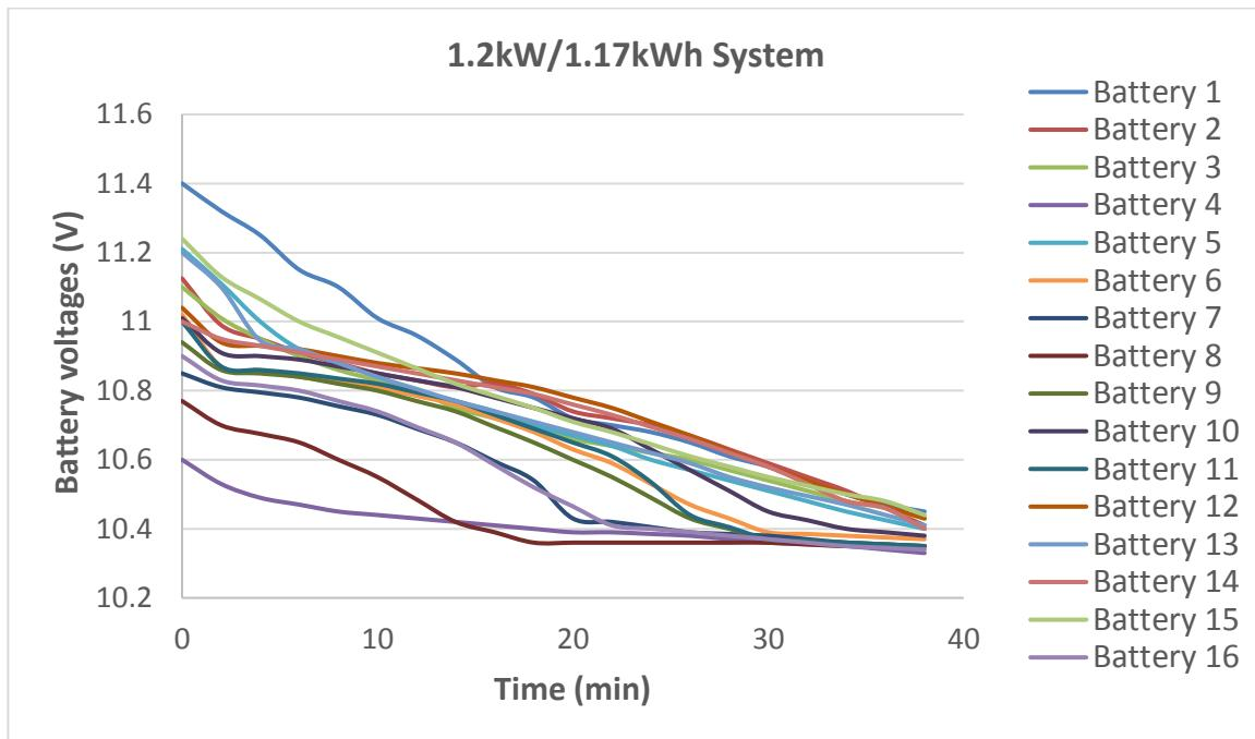
Fig. 43. Terminal voltage uniform result during discharge process.
