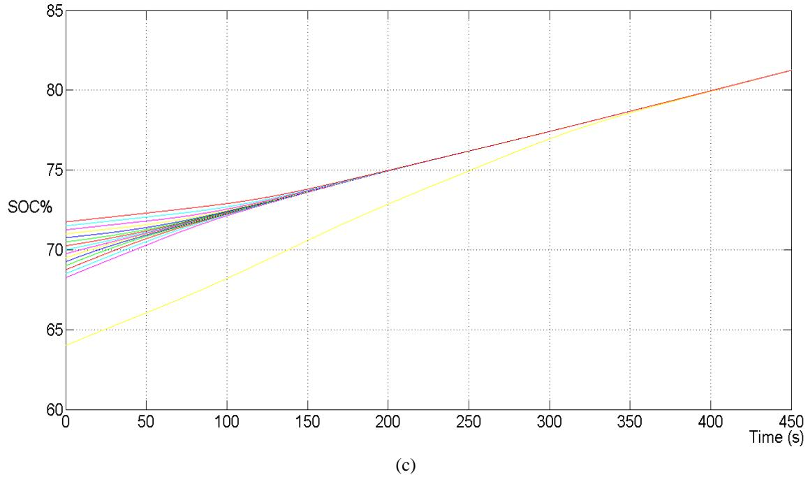
Fig. 39. SOC balancing of modules during charging process: (a) phase A, (b) phase B, and (c) phase C.
