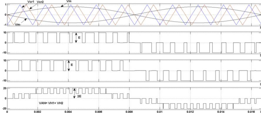
Fig. 18. Five-level CHB inverter with phase-shifted PWM modulation scheme ( $m=0.8$ ,  $m_f=10$ ,  $f_{cr}=600$  and  $f_m=60$  Hz).
