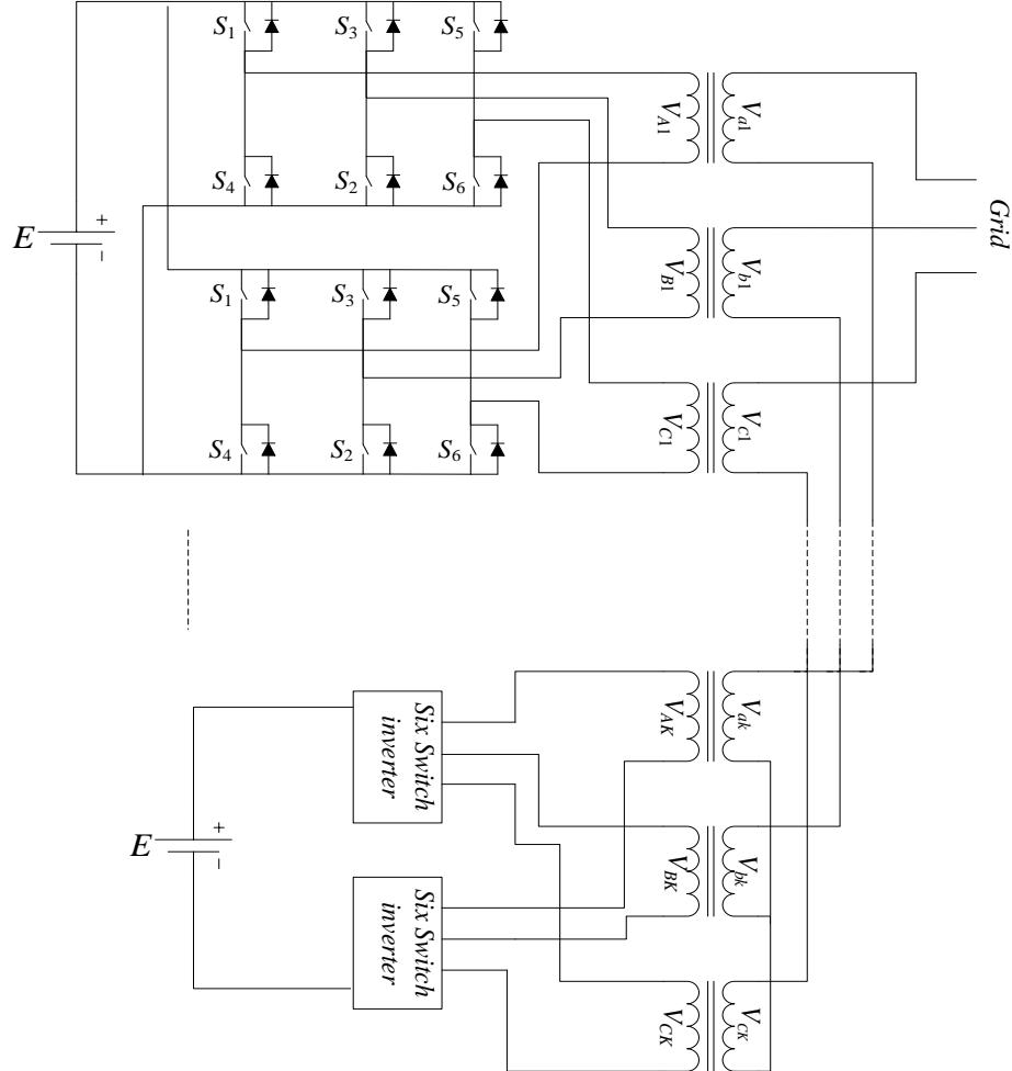
Fig. 21. Circuit topology of the SSCT inverter.
