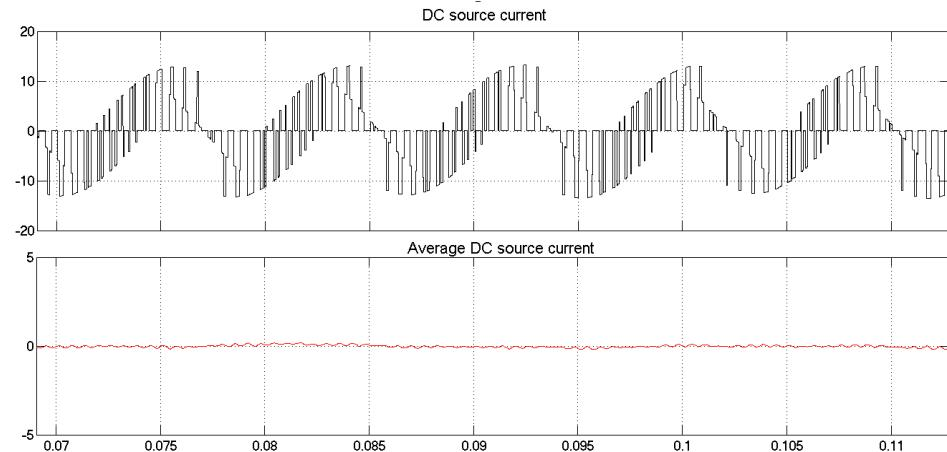
Fig. 49. DC source current of the SSBC circuit.
