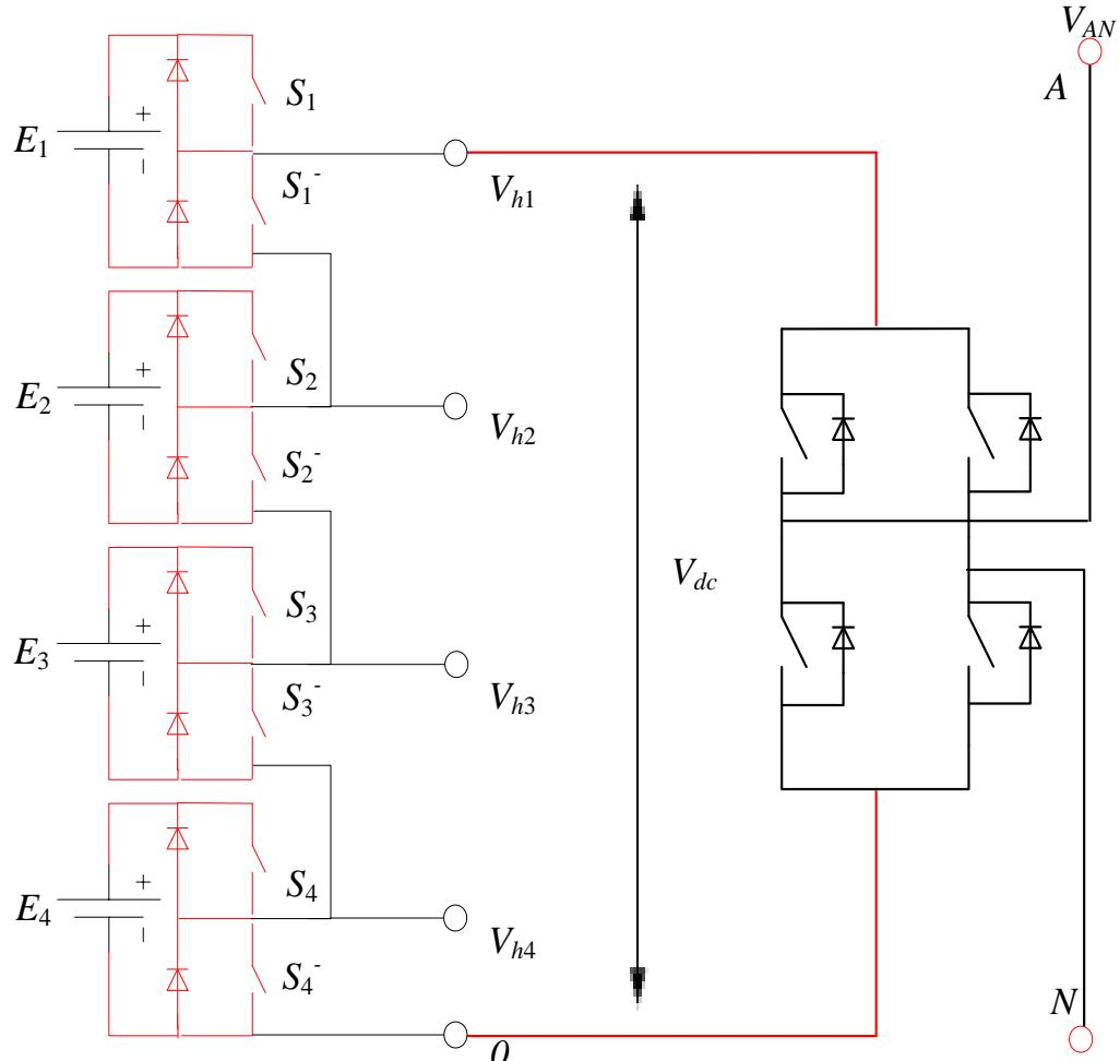
Fig. 28. Topology of a single-phase nine-level HCMC inverter.
