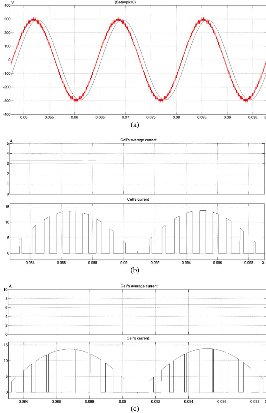
Fig. 35. Discharging process: (a) 33-level HCMC inverter and grid  $V_{L-L}$  waveforms (fundamental frequency= 60Hz, and carrier frequency= 600Hz), (b) A module with a low SOC ( $m_{i,x}=0.5$ ), (c) A module with a high SOC ( $m_{i,x}=0.97$ ).
