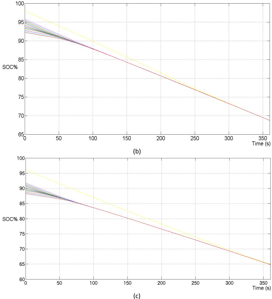
Fig. 38. SOC balancing of the battery modules during the discharging process: (a) Phase A, (b) Phase B, and (c) Phase C.
