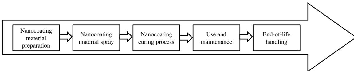
Figure 2.3. The life cycle of nanocoating material.
