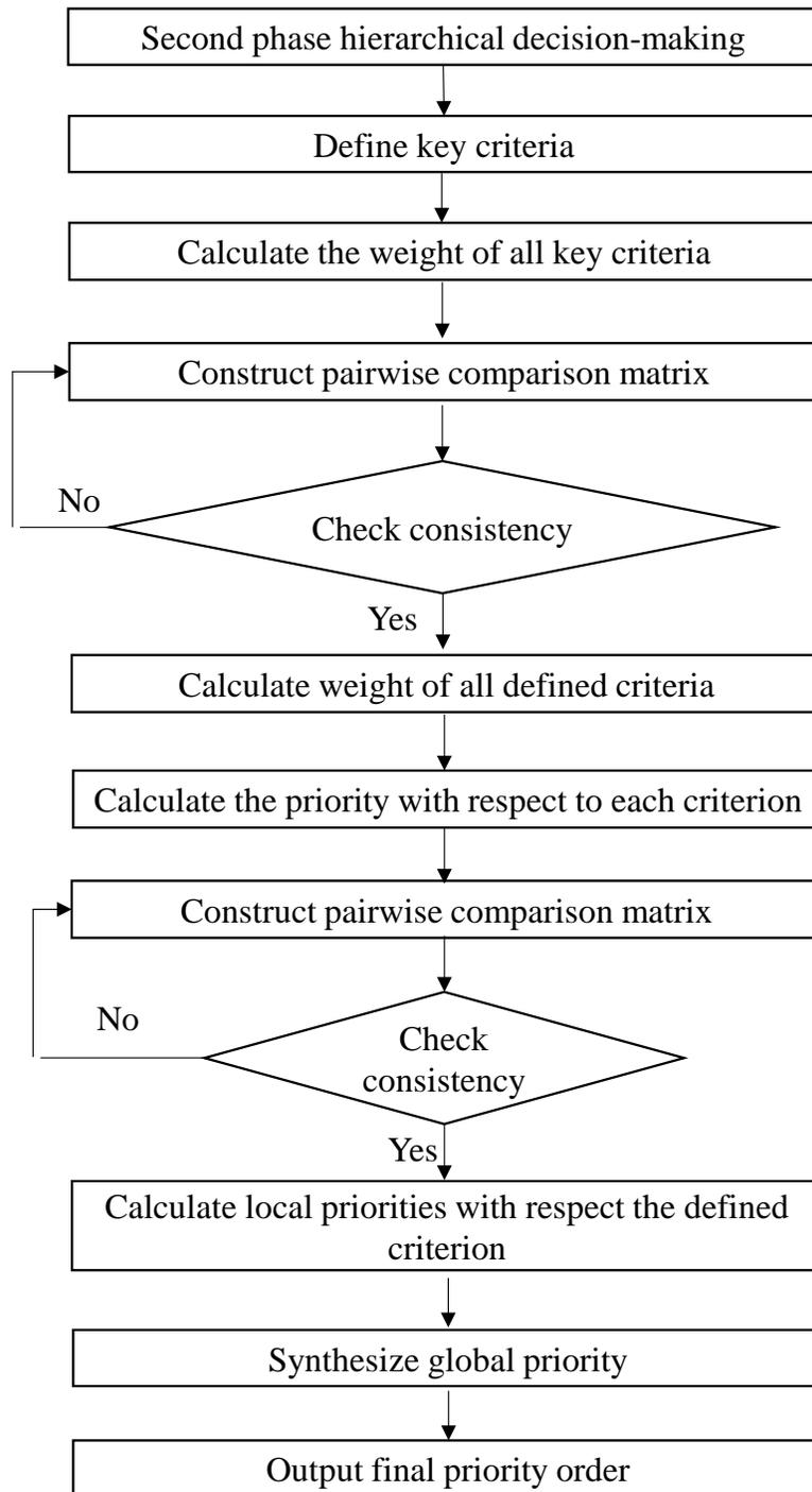
Figure 3.6. General scheme of AHP based prioritization process.
