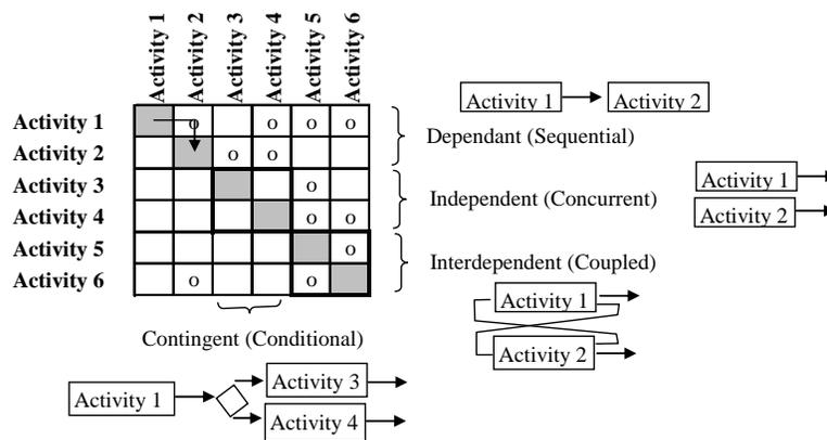
**Figure 2-1: Design Structure Matrix** (Browning, Co, 2001)
