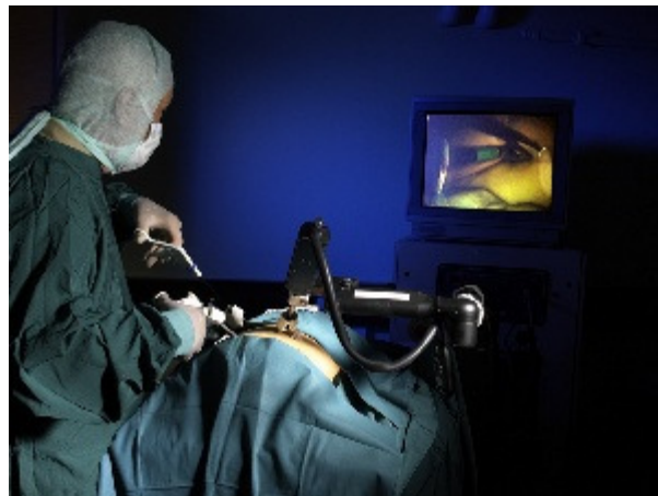
Figure 2 Surgeon performing a laparoscopic surgery with the computer vision guided camera control system similar to the one used Universitat Politècnica de Catalunya
