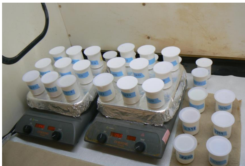
Figure 2.15. Electroplating of ^{210}\text{Po} on to polished silver planchets.
