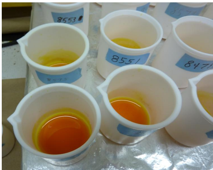
Figure 2.18. Residual solution dried before taking to 9M HCl for anion exchange column.
