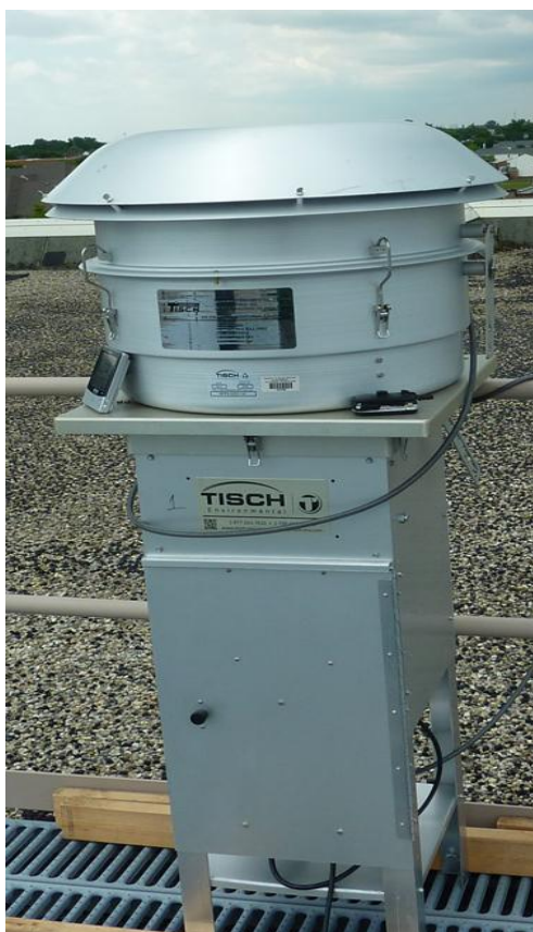
Figure 2.22. High-Volume Tisch Environmental TSP TE5170V aerosol sampler.
