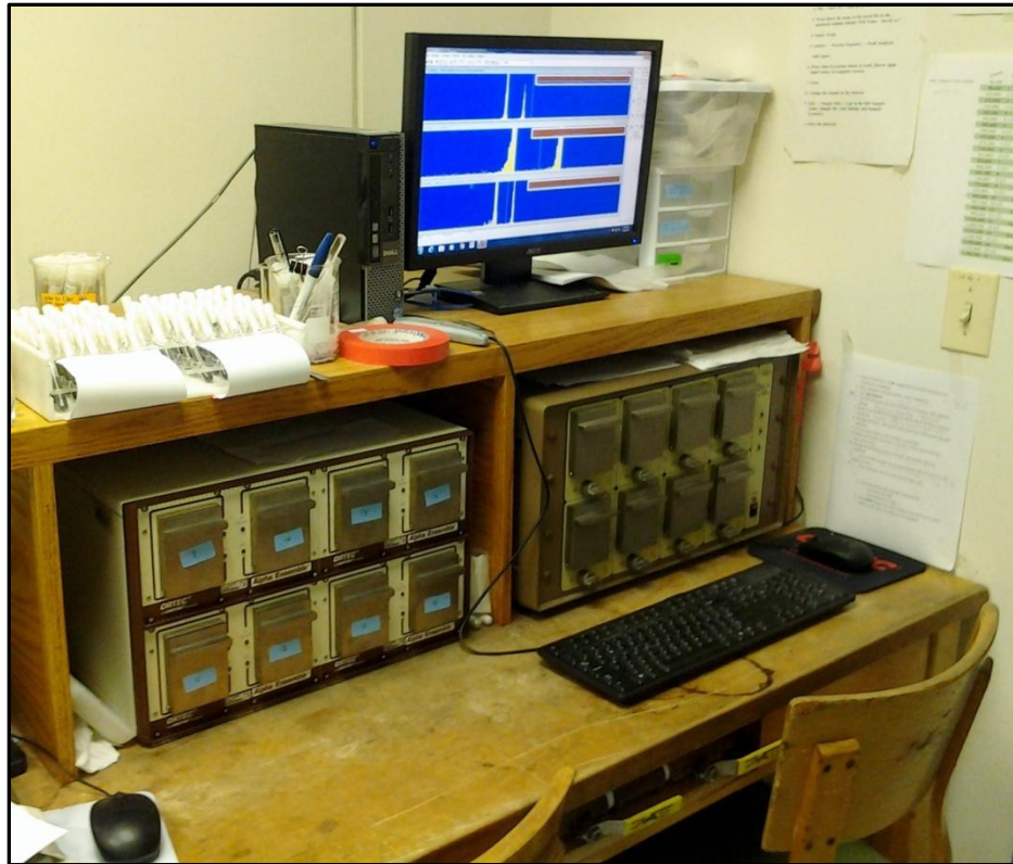
Figure 2.16. Silver planchet analyzed in (16) Octete PC 8-input alpha spectrometers.
