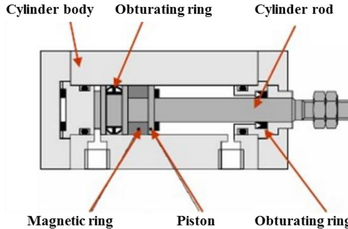
Figure 19 The structure and components of the traditional air cylinder.
