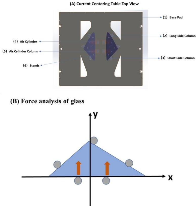
Figure 8(A) a schematic of the structure of the current centering table and (B) A schematic of the force analysis of glass on the centering table.
