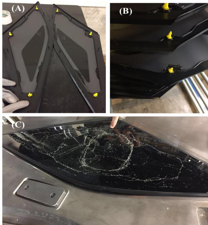
Figure 10 Low quality of the glass fabricated by the current centering table. (A) injection flash because of dislocation in the centering table, (B) large deviation, (C) chunk glass in the mold because of dislocation in the centering table.
