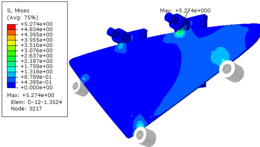
Figure 17 The stress distribution on the glass on static state with an impetus of 80N.
