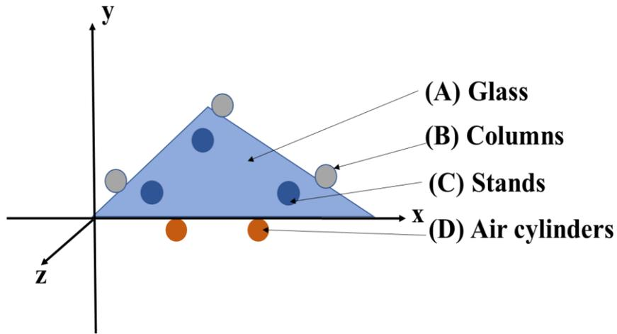
Figure 7 The columns and air cylinders needed on the centering table to constrain the glass and remove the DOF of the glass.
