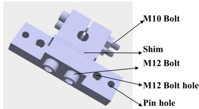
Figure 22 The structure of the new design of the column base.
