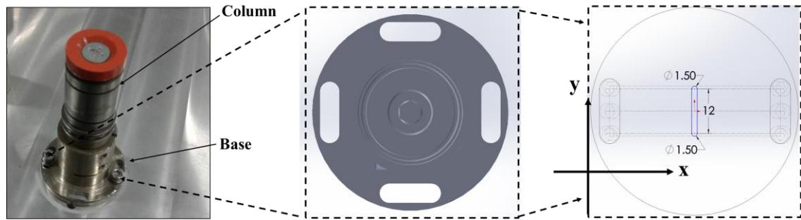
Figure 9 The structure of the column base on the current centering table.
