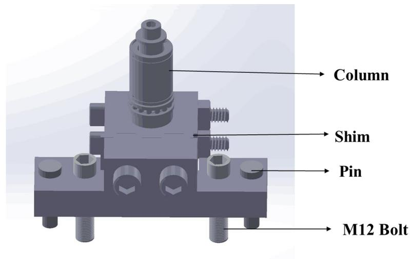
Figure 23 The schematic of the column base after assembling the column.
