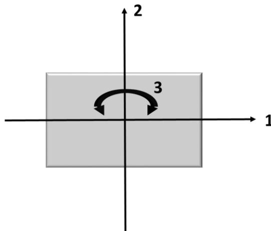
Figure 5 A rigid body in an x-y plane with 3 degrees of freedom.
