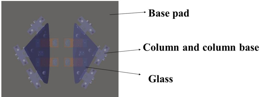
Figure 24 The new design of the centering table which contains six columns.
