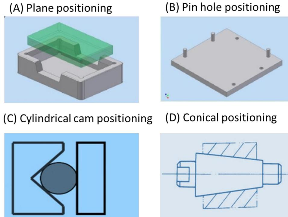
Figure 6 Schematic of the four basic positioning mechanism.
