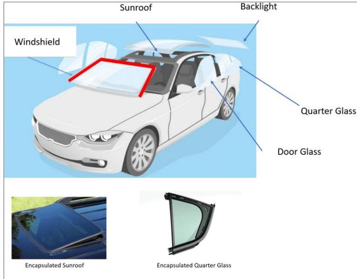
Figure 2 Schematic of the encapsulated quarter glass and a car.
