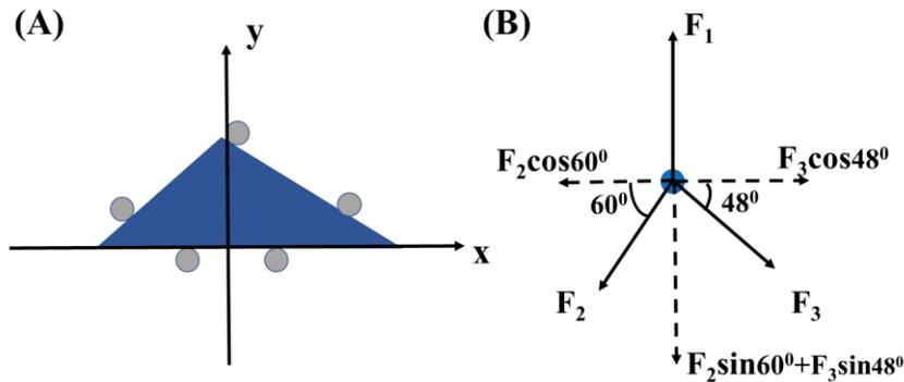
Figure 18 (A) The relative position of the glass and the columns. (B) The force analysis of the glass under the pressure of columns on the centering table.
