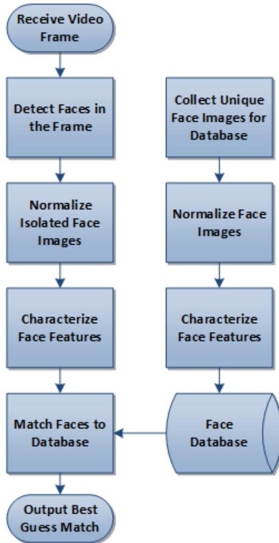
**Figure 2.1: Process for Performing Face Recognition**
