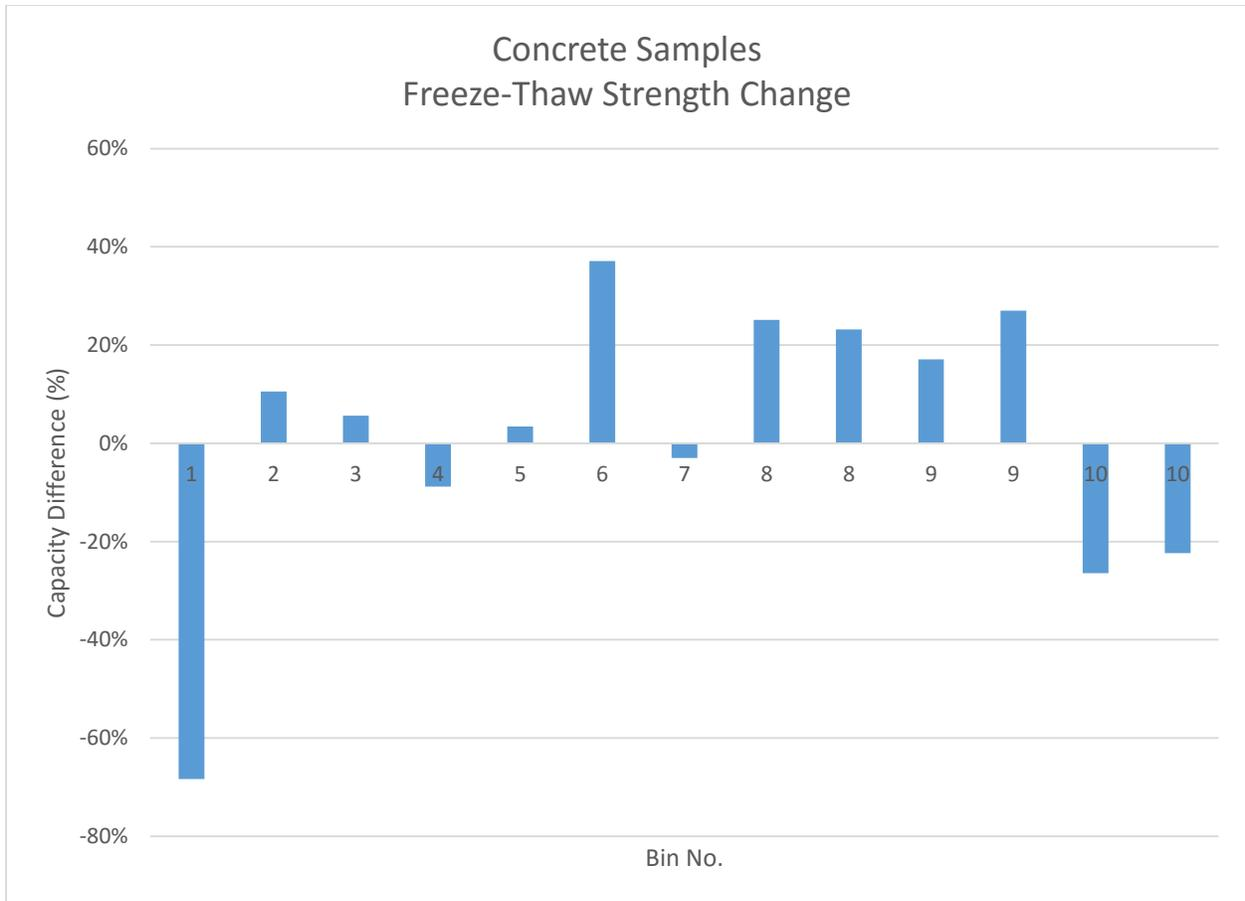
Figure 35: Strength change in concrete samples after freeze-thaw cycling.
