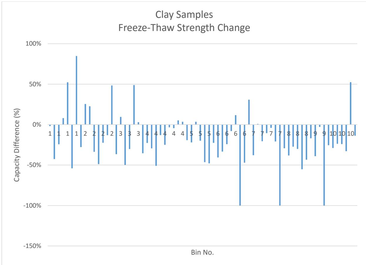
Figure 33: Strength change in clay brick samples after freeze-thaw cycling.
