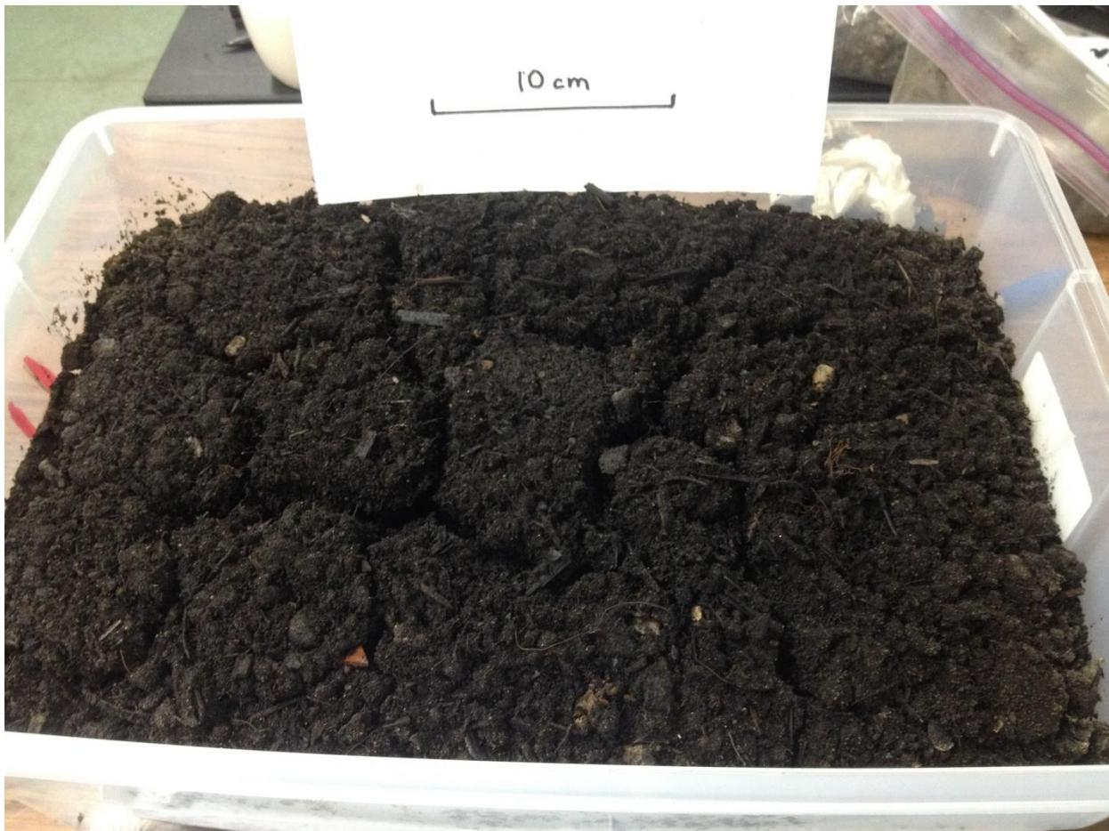
*Figure 19: Close up of large fissures and weak granular structure developed in Bin No. 4.*
