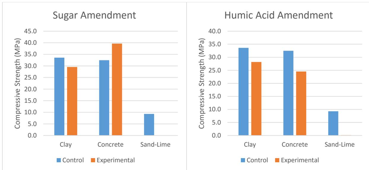
Figure 36: Plots of control strength values versus experimental strength values for all samples and all amendments.
