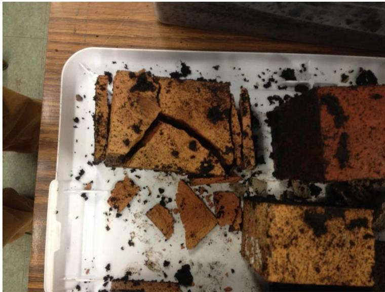
*Figure 29: Brick sample broken in situ during freeze-thaw cycling.*
