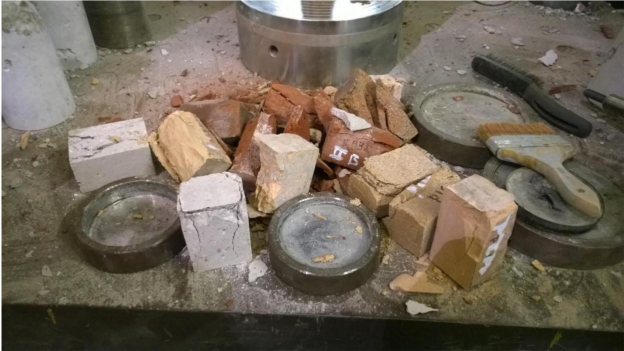
*Figure 18: Samples after compressive strength testing.*
