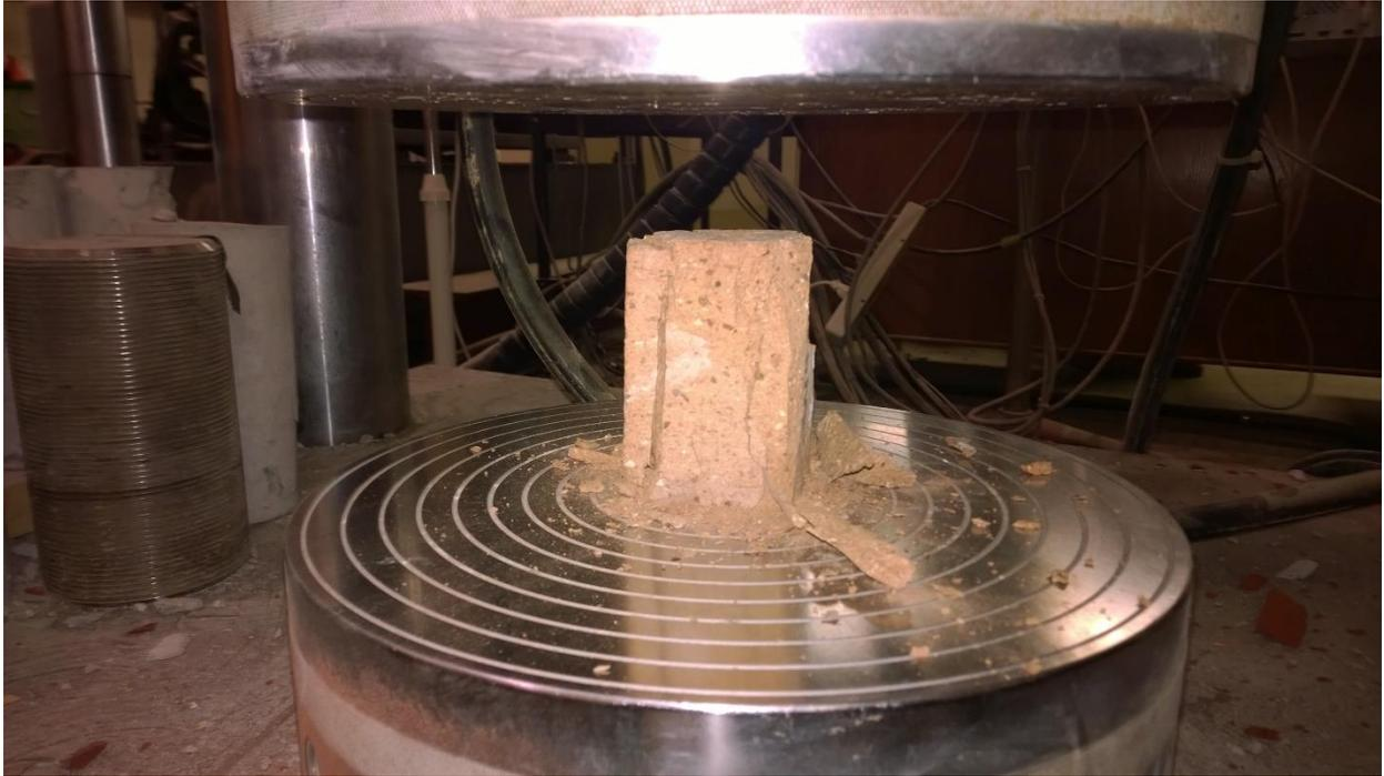
*Figure 17: Brick sample that has undergone uniaxial compression testing.*
