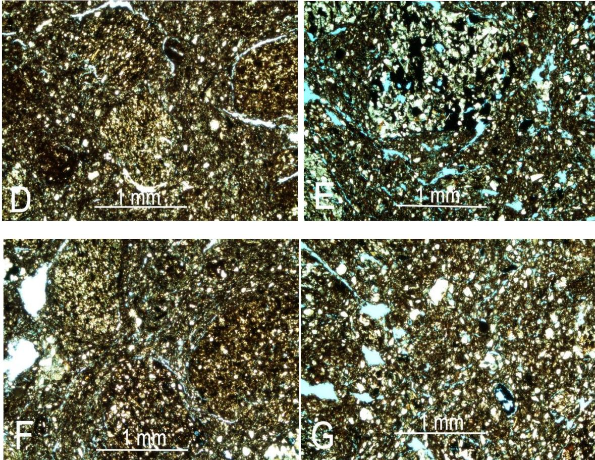
Figure 37: Photomicrographs of brick sample thin sections as a function of treatment. A, concrete control; B, concrete with sugar treatment; C, concrete after NaCl treatment; D, Brick type 1 control; E, Brick type 1 after sugar treatment; F, Brick type 2 control; G, Brick type 2 after NaCl treatment.
