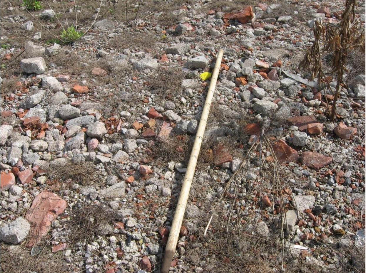
*Figure 4: In the past, some contractors prepared a demolition site for future building construction by intentionally leaving a large volume of rock-like artifacts to form what they called "hardcore." Staff is marked in 10 cm intervals.*
