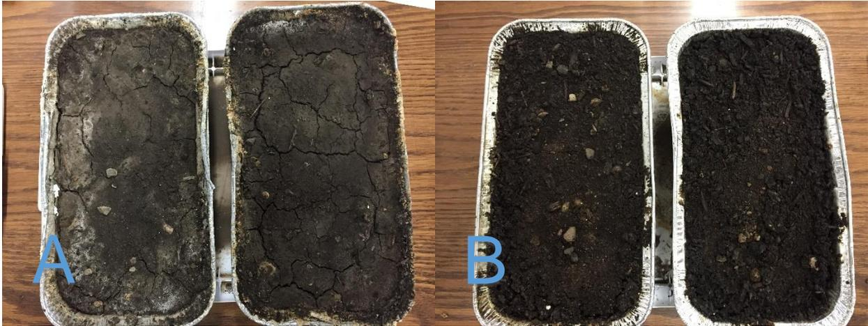
Figure 21: A, Interconnected fissures in the soil surface developed in the bin treated with a salt solution; B, Weak granular structure developed in the bin treated with a sugar solution.
