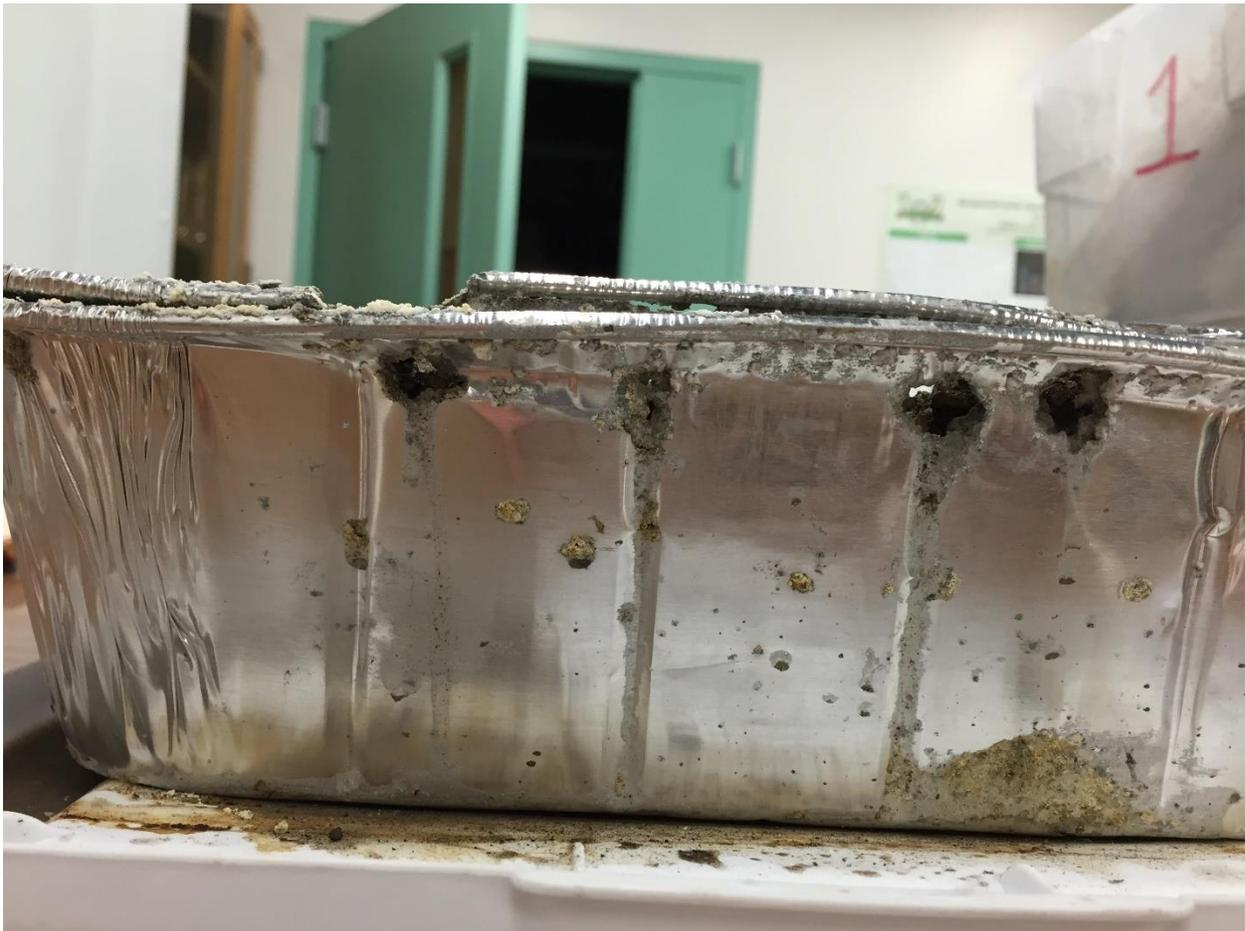
Figure 22: Corrosion of the aluminum pan treated with salt solution.
