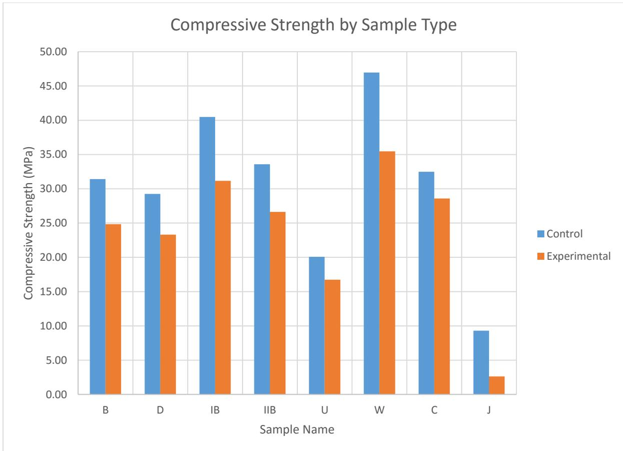
Figure 31: Compressive strength for all tests, by sample type.
