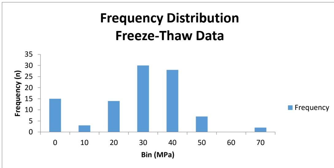
Figure 28: Frequency distribution of all post-weathering compression testing data.
