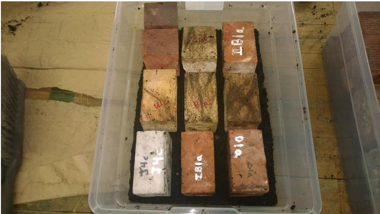
*Figure 14: Example showing arrangement of brick samples in simulated soil.*
