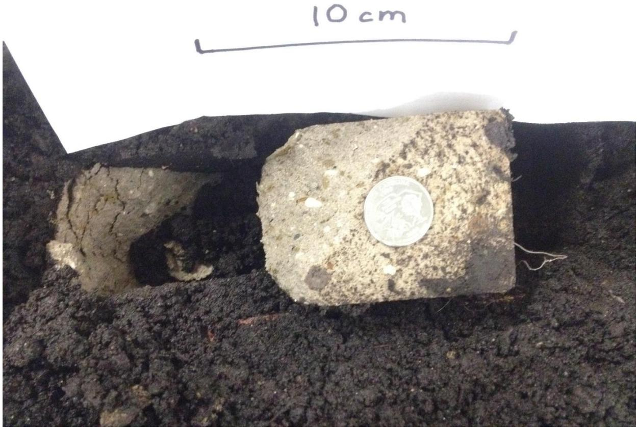
*Figure 23: Severe physical breakdown of a sand-lime brick sample.*
