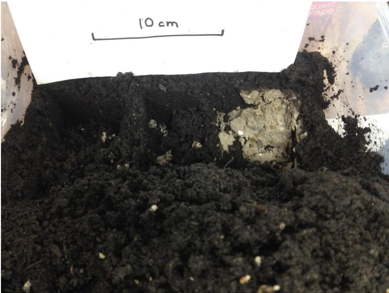
*Figure 24: Spalled pieces of sand-lime brick after freeze-thaw cycling.*
