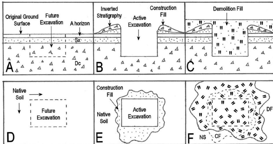
Fig. 9. Genetic model showing how construction and demolition processes affect demolition site stratigraphy and anthrosequence development: A, Residential site prior to construction; B, Inverted stratigraphy resulting from excavation for basement; C, Stratigraphy following demolition and backfilling. D, E, and F are map views of A, B and C, respectively. NS, native soil; CF, construction fill; DF, demolition fill; Sx, glaciolacustrine sand capping; Dc, clayey diamicton.
