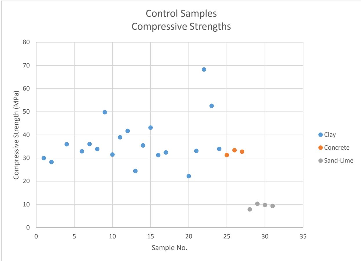
Figure 26: Scatterplot showing compressive strengths for control samples.
