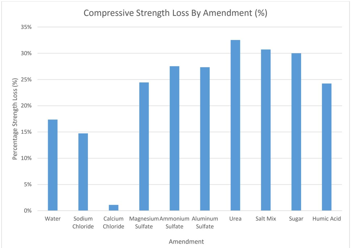
Figure 30: Compressive strength loss by amendment.
