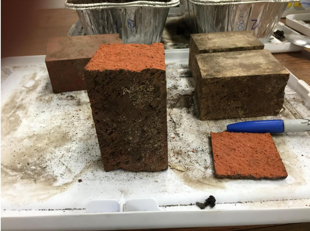
*Figure 25: Spalled brick sample removed from salt wet-dry experiment*
