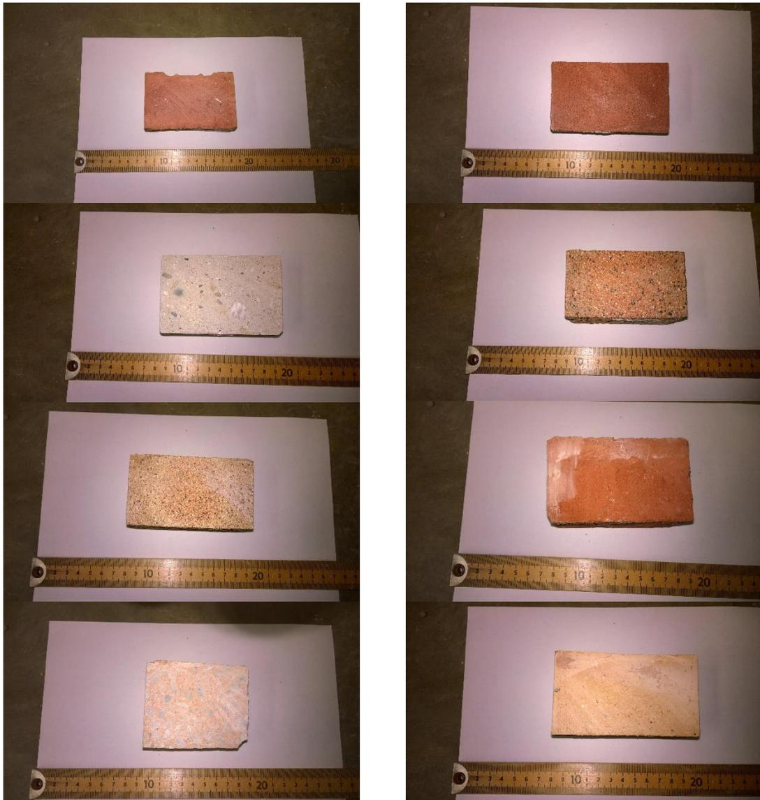
*Figure 12: Cut brick samples used for the simulated weathering experiment.*
