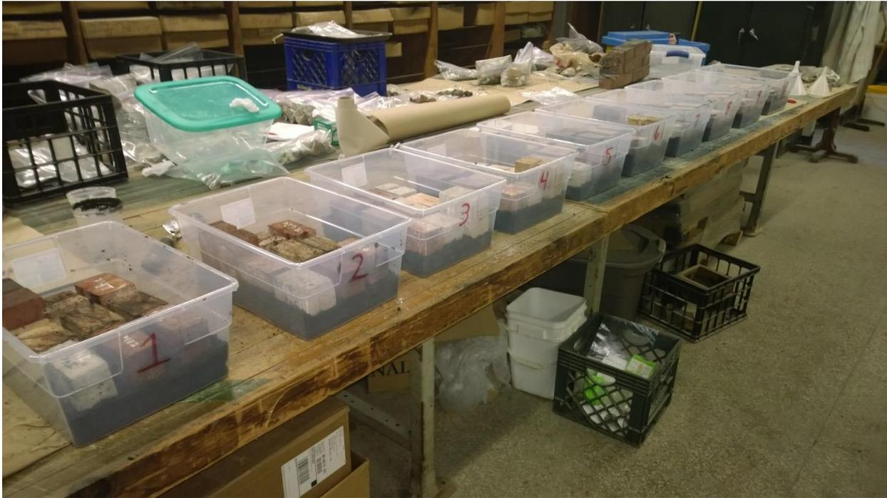
*Figure 13: Ten plastic bins with brick samples partially buried in topsoil.*
