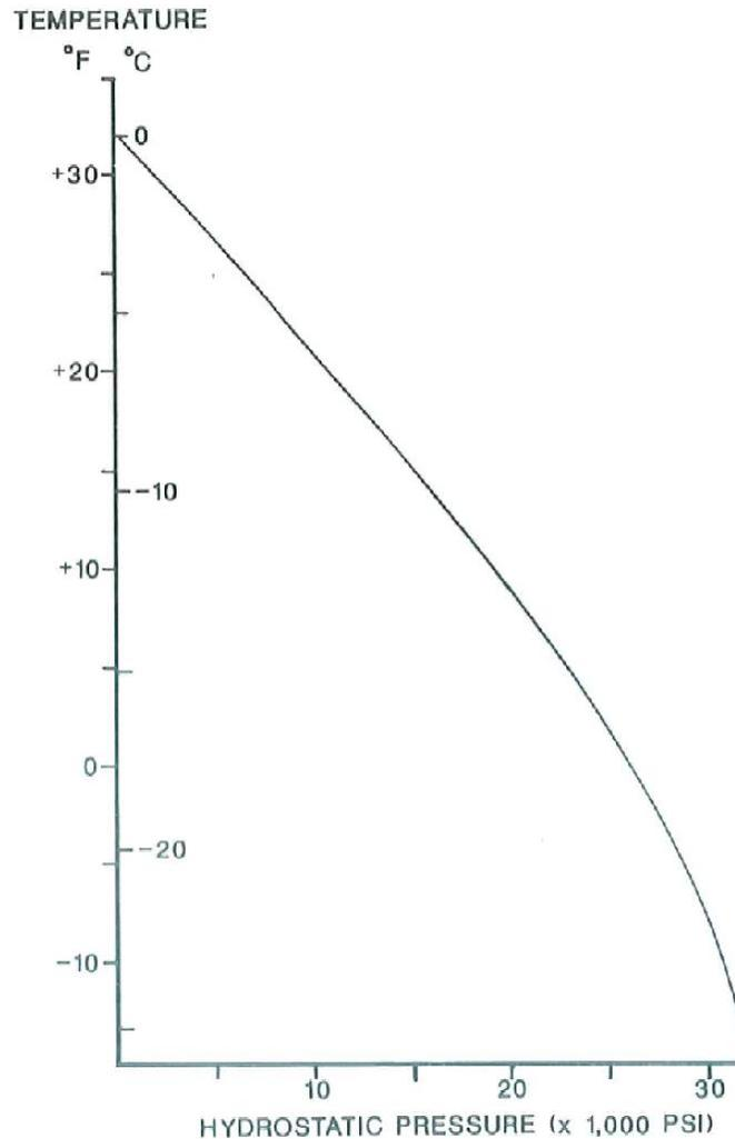
Figure 10: Hydrostatic pressure versus temperature in a closed system, taken from Lienhart 1988
