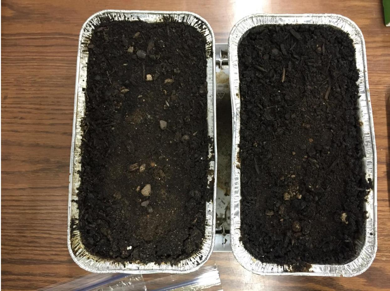
*Figure 16: Wet-Dry experimental set up (sugar solution)*
