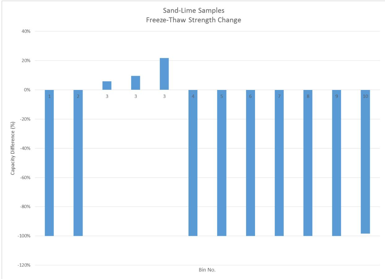
Figure 34: Strength change in sand-lime samples after freeze-thaw cycling.
