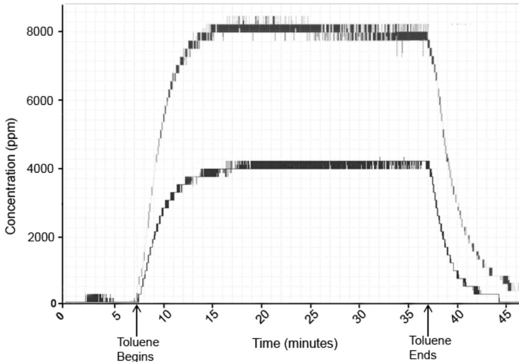
*Figure 3:* Infrared spectroscopy plot of increasing and decreasing toluene concentrations within the dynamic exposure chamber. Each vertical line represents one min. Toluene concentration reached the target 4000 ppm or 8000 ppm in approximately 7.5 min and remained constant until exposure was discontinued at thirty min. Evacuation of toluene from the chamber took between 7.5 and 9.5 min, depending on the dose utilized.
