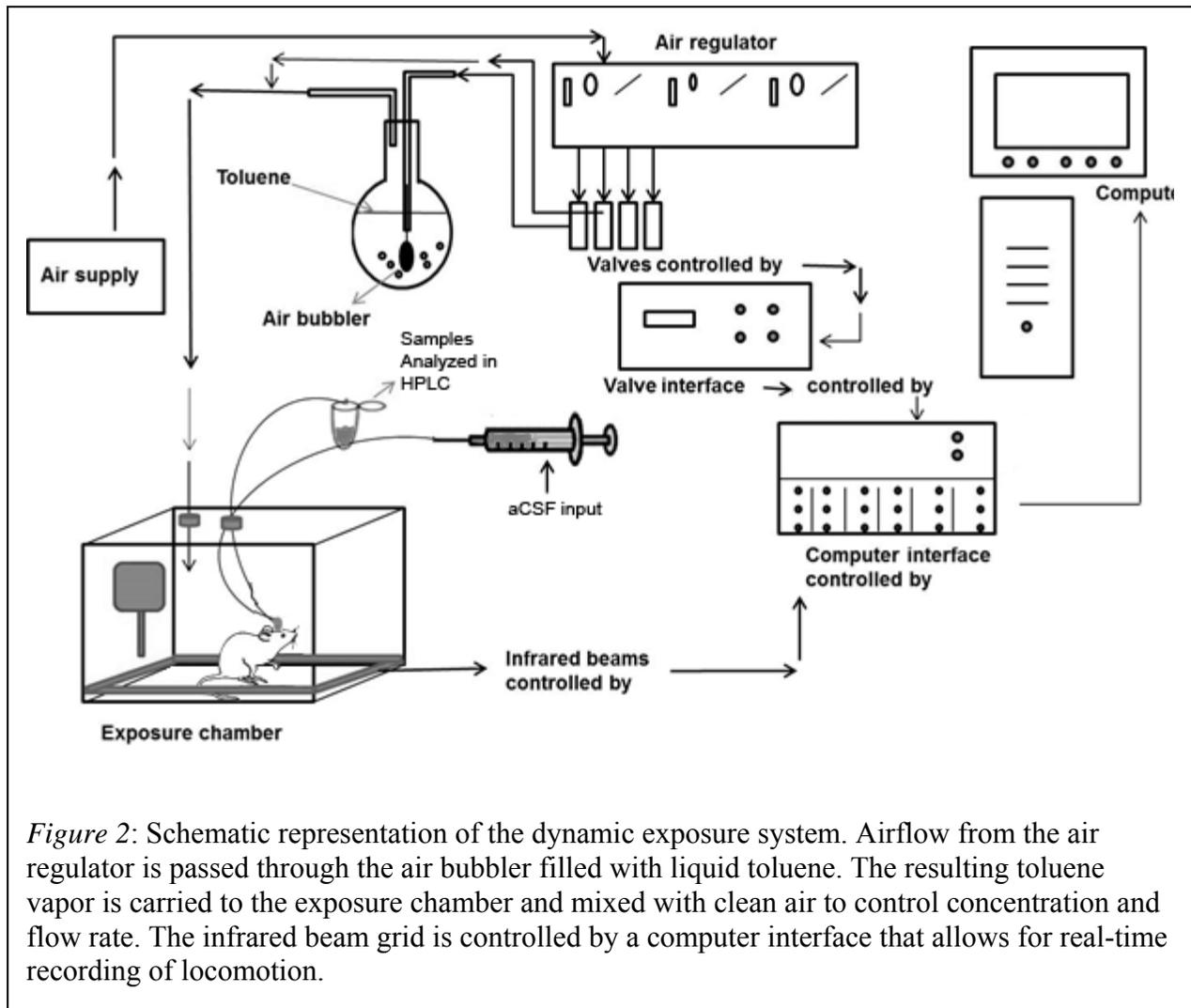
*Figure 2:* Schematic representation of the dynamic exposure system. Airflow from the air regulator is passed through the air bubbler filled with liquid toluene. The resulting toluene vapor is carried to the exposure chamber and mixed with clean air to control concentration and flow rate. The infrared beam grid is controlled by a computer interface that allows for real-time recording of locomotion.
