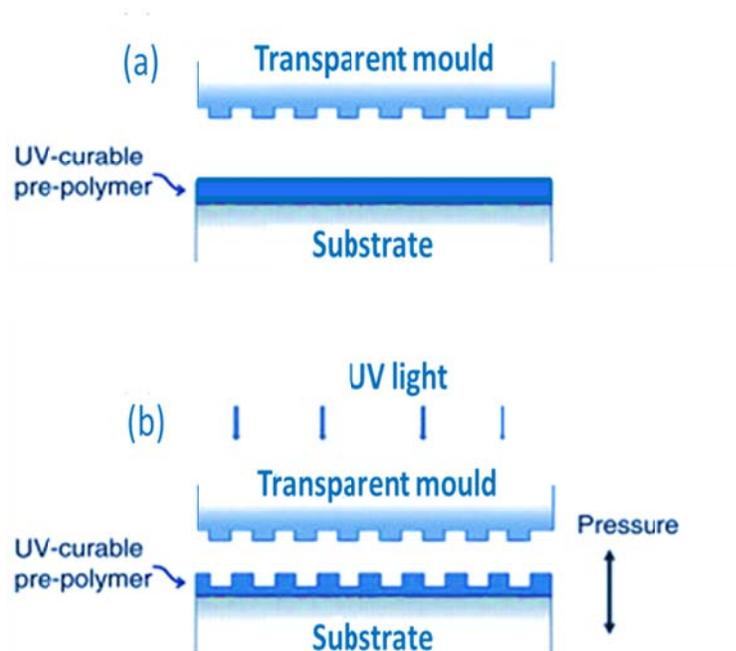
Figure 3.2: Schematic illustration of UV NIL. (a) The substrate is coated by a UV-curable liquid polymer resist. (b) A transparent mould (quartz glass) is pressed into the substrate. The imprinted nanostructures are cured by UV-radiation applied to cross-link the polymer resist and to facilitate pattern formation on the substrate at room temperature and under reduced pressure (0-5 bar). Subsequently, the mould is released leaving the imprinted structures on the substrate. Adapted from [11]
