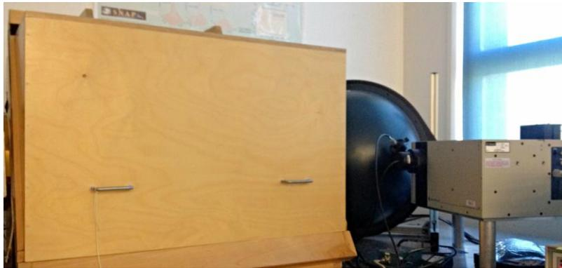
Figure 4: The light uniformity section, connected from right to left: monochromator, integrating sphere, black box.
