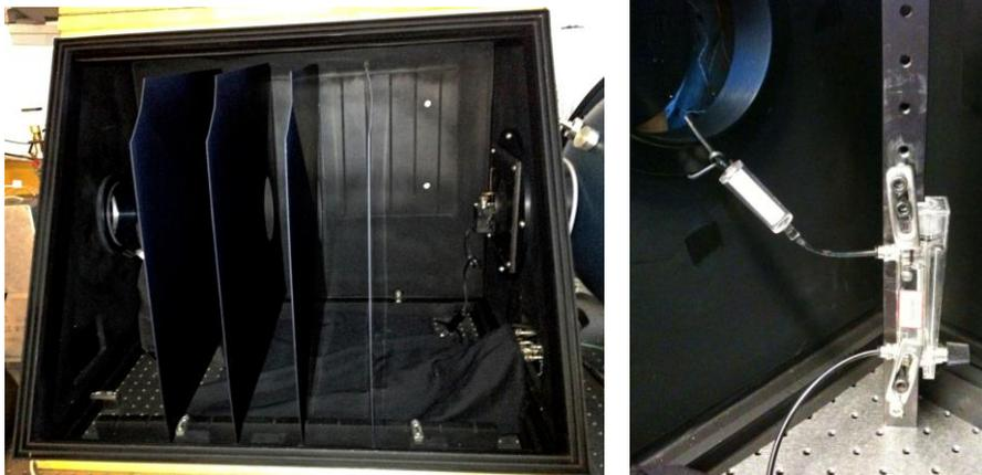
Figure 7: Left: the interior of the black box (developed by Don Groom). The Dewar is connected on the left and a shutter connected to the integrating sphere is connected on the right. Right: compressed air delivery apparatus used to remove condensation from the window when the Dewar is cold.
