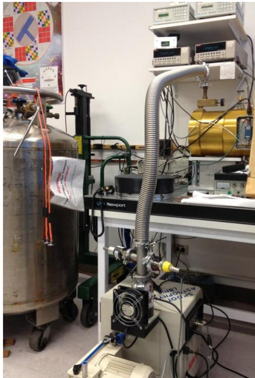
Figure 8: The Dewar and photodiode container section. From right to left: the Dewar and controller. Above are two Keithley Picoampmeters and two Lakeshore temperature controllers. On the left is the liquid nitrogen container that is used to fill the Dewar. Below is the vacuum pump.
