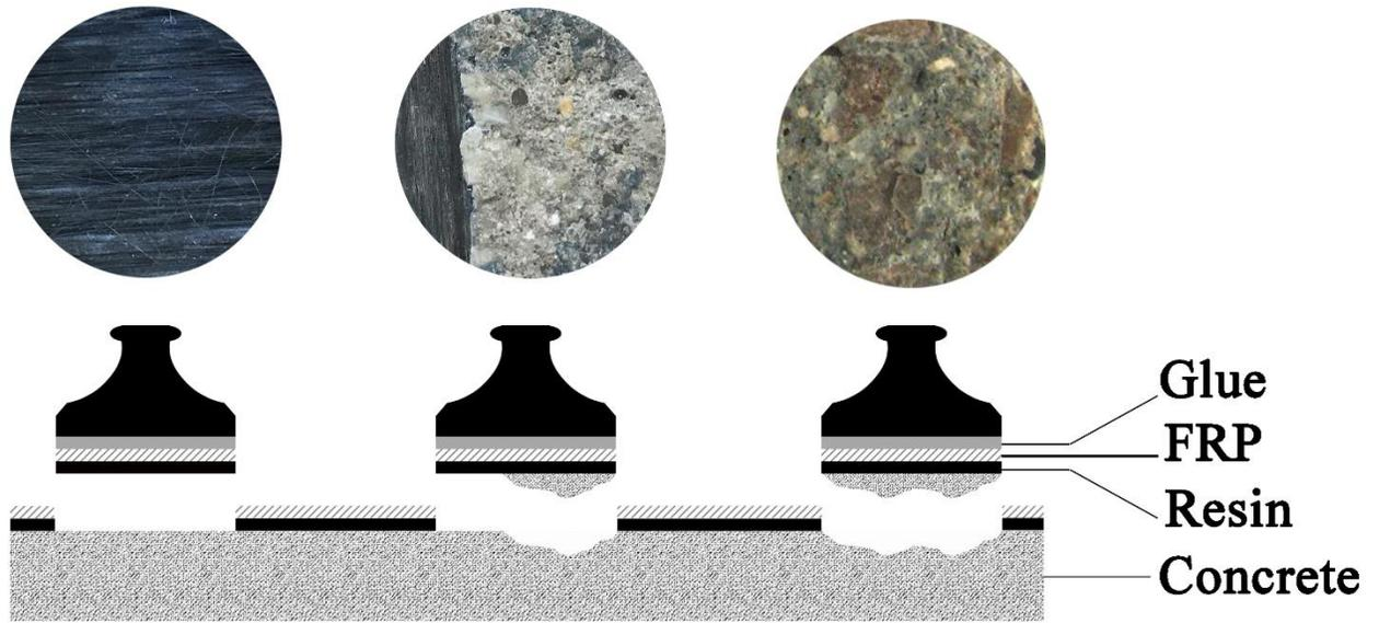
**Fig. 3.** Pull-off Test Failure Modes: (a) FRP adhesive failure; (b) Mixed concrete/FRP failure; (c) Concrete substrate failure
