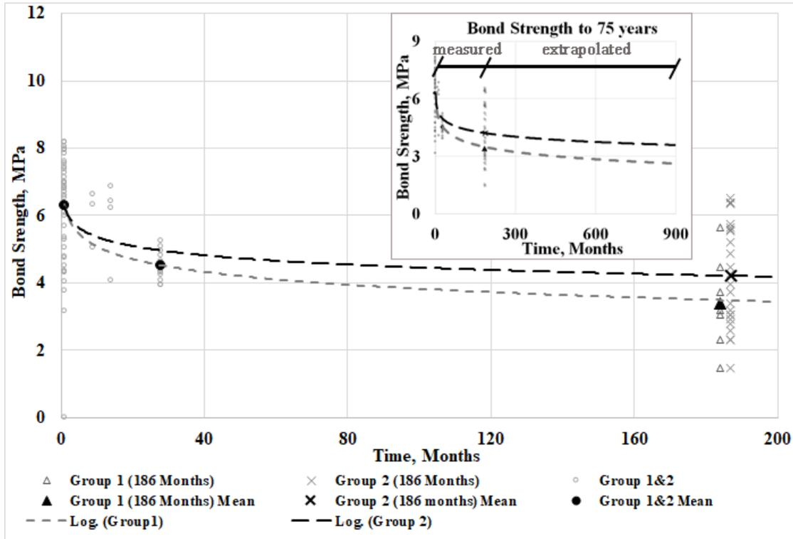
**Fig. 5.** Bond Strength as a Function of Weathering Time.
