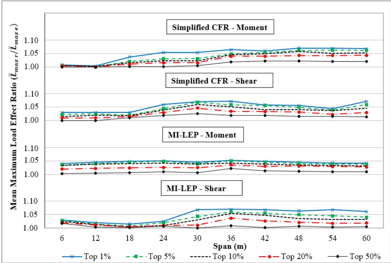
Figure 6. Effect of Database Reduction on Mean Maximum Load Effect.
