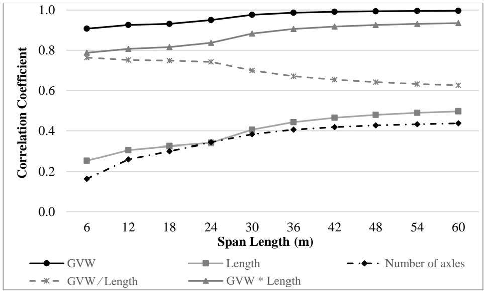
Figure 2. Correlation Between Vehicle Parameter and Moment, Simplified CFR.
