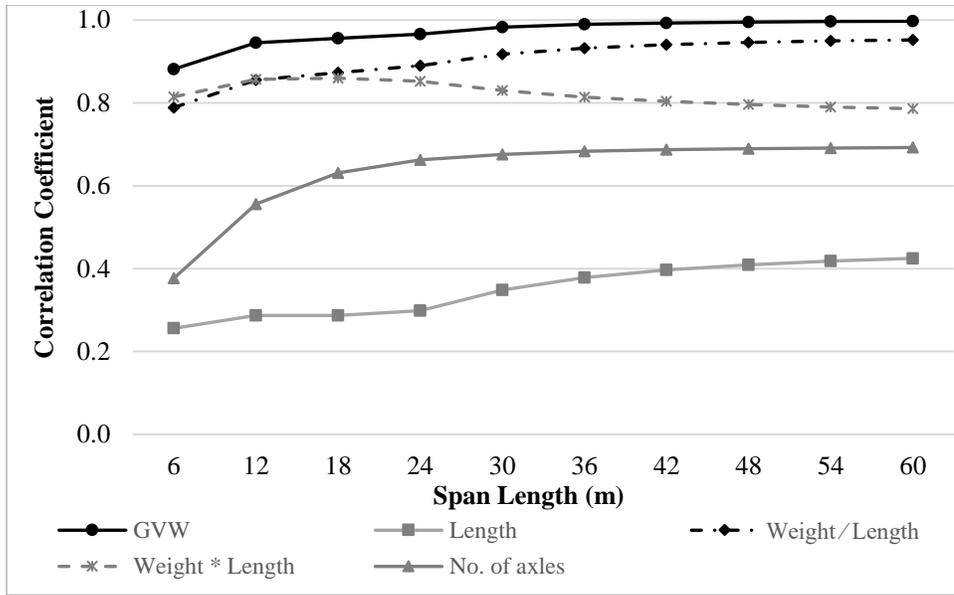
Figure 1. Correlation Between Vehicle Parameter and Moment, MI-LEP.
