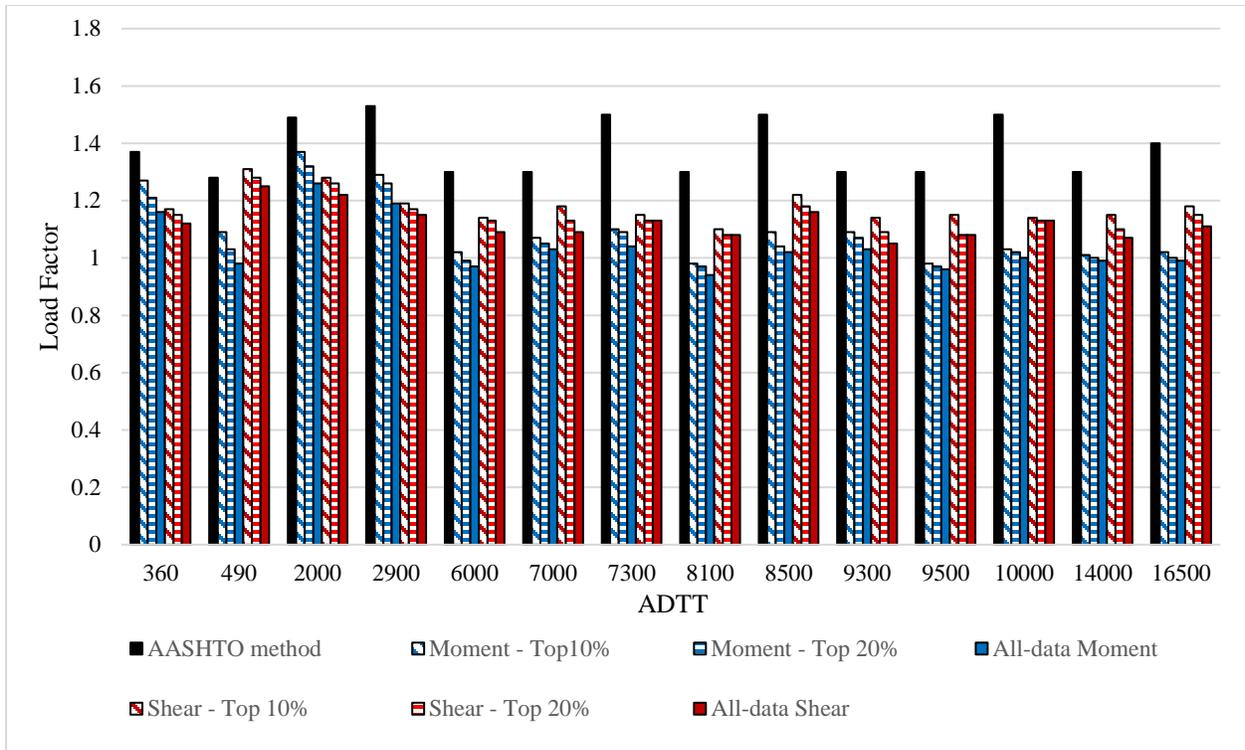
Figure 9. Comparison between AASHTO and Proposed Procedure, Simplified CFR.
