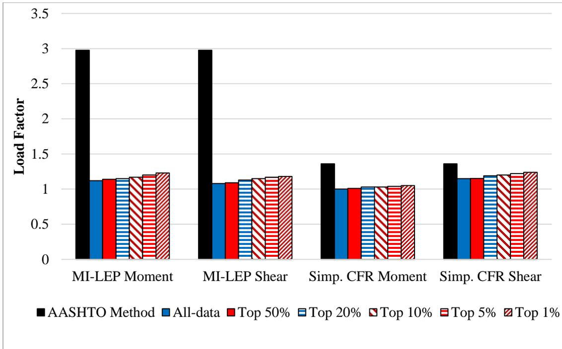
Figure 7. Comparison between AASHTO and Proposed Procedure.
