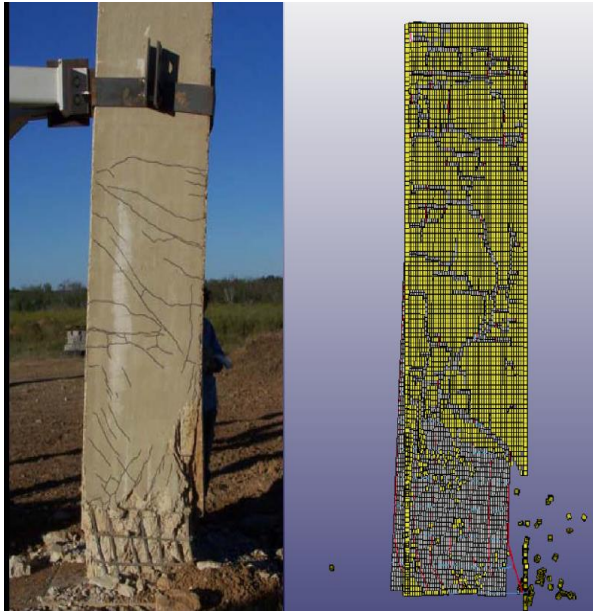
Figure 4. Comparison of Experimental and FEA Results (Alsendi and Eamon 2020; Williamson et al. 2011).
