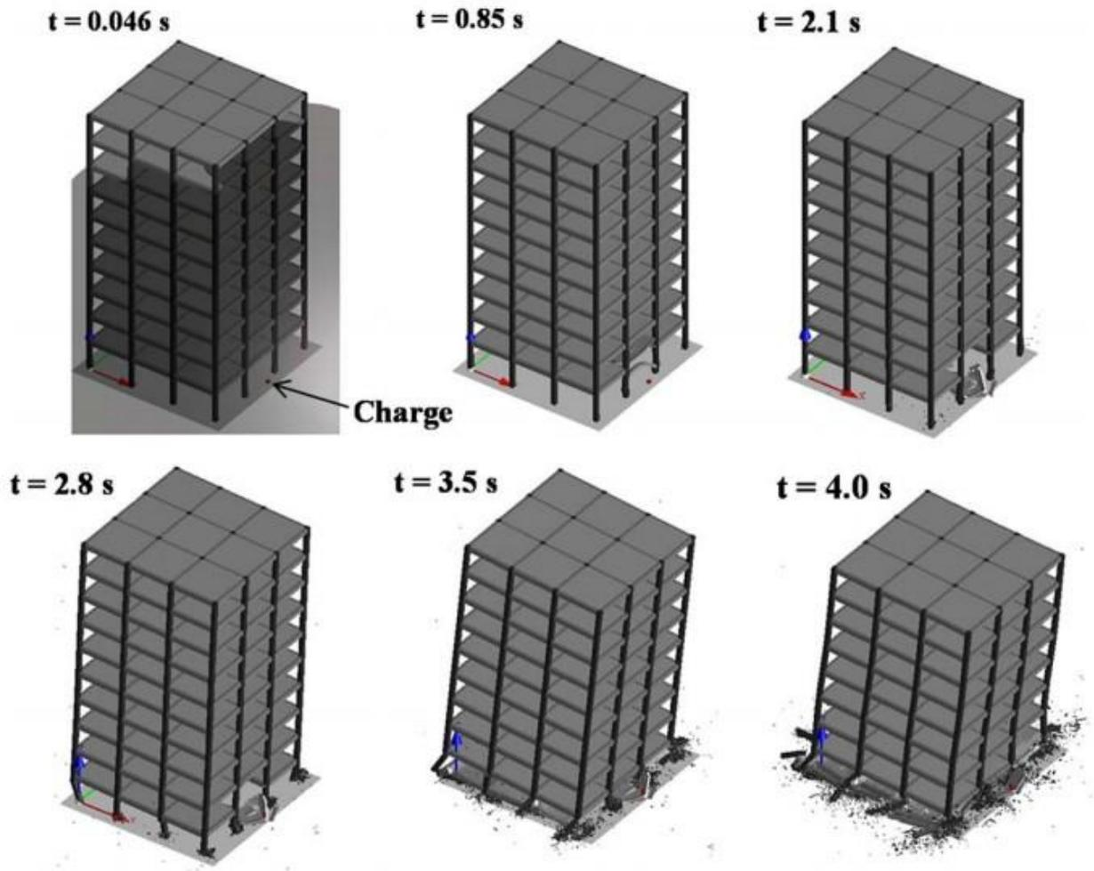
669 **Fig. 6.** Response of 3x3 MRF Structure
