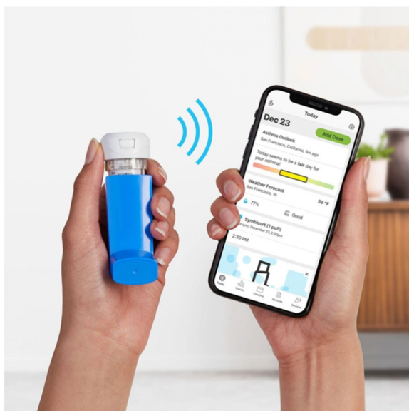
Fig. 1 The digital self-management platform included a medication sensor to capture inhaler use and a companion smartphone app to receive medication reminders and education
