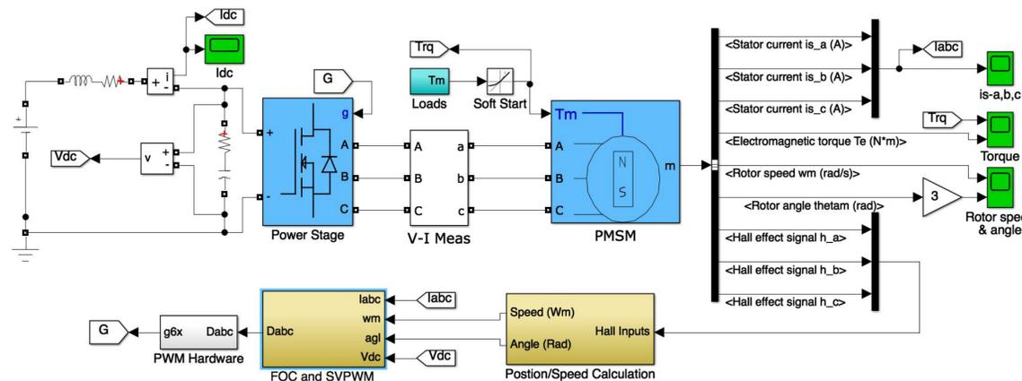
**Fig. 2** MATLAB/Simulink motor drive simulation with hall sensor interpolation algorithm.
