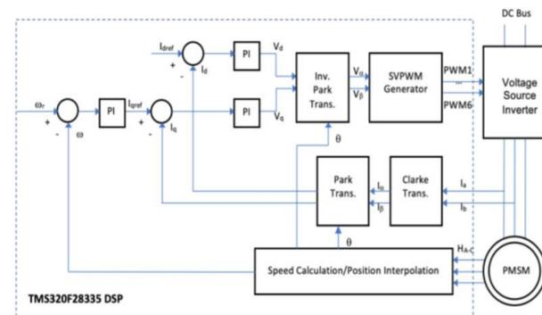
**Fig. 1** Block diagram of the FOC control strategy.
