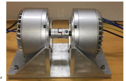
**Fig. 4.** Motor drive test bed
