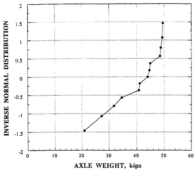
Fig 1. Cumulative Distribution Function of Maximum Axle Weight
