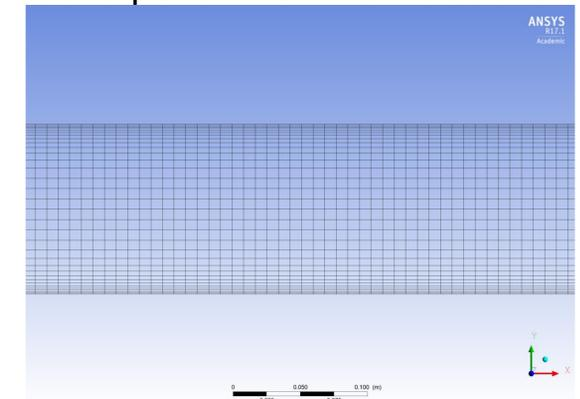
Fig. 2. Example of mesh for a reforming tube. Grid spacing is tighter near the walls.
