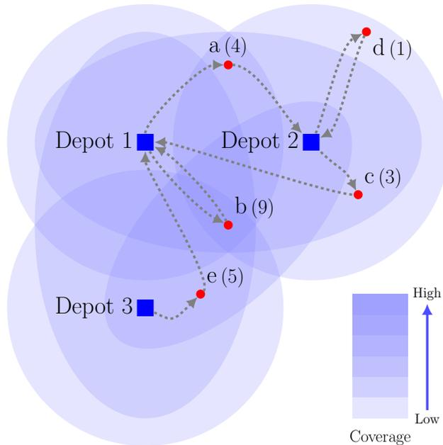
Figure 1: A drone delivery service area having three depots and five customer locations. Customer  $e$  is serviceable by 5 delivery routes while customer  $d$  is serviceable by only one route. In this paper, we require all customers to be serviceable by at least 3 routes, i.e., covered by an ellipse.
