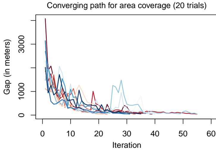
Figure 11: Convergence pattern of the area coverage algorithm applied to Troy with  $p = 6$  depots.
