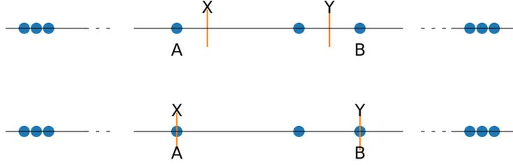
Figure 7: Upper: The two nearest depots,  $X$  and  $Y$ , to the demand point  $A$  both fall on the right side of  $A$ . This is not a regular solution, and can be changed to a regular solution (Lower) without affecting the objective value.
