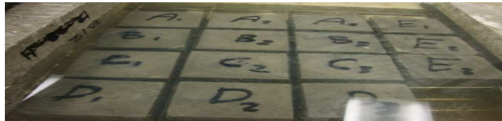
Figure 4.1: Freeze thaw tray loaded with specimens
