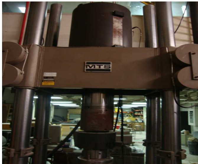
Figure 4.4: MTS 810 machine employed for compression test
