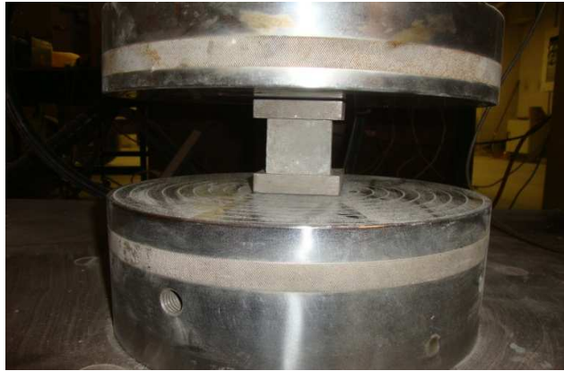
Figure 4.5: Compression test setup of a prism specimen
