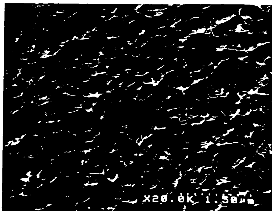
Fig. 2.3.3.1 The SEM micrograph of the graded down film.
