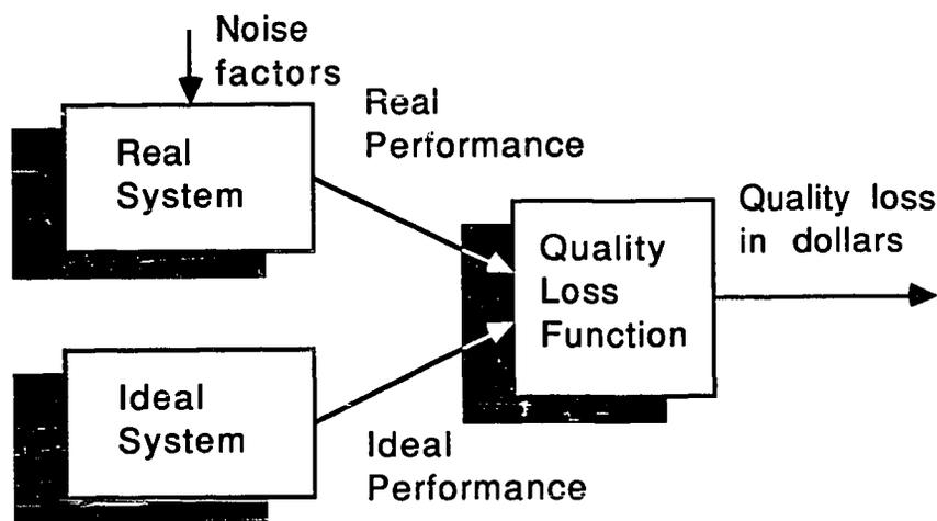
Figure 2.1. QLF transfers deviations to a quality loss in dollars.
