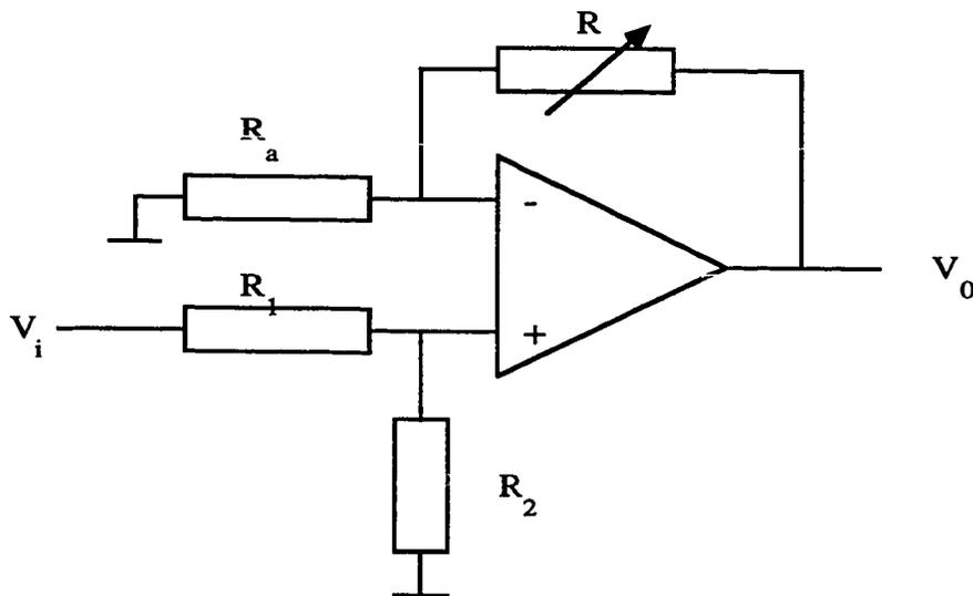
Figure 4.4. A noninverting amplifier.
