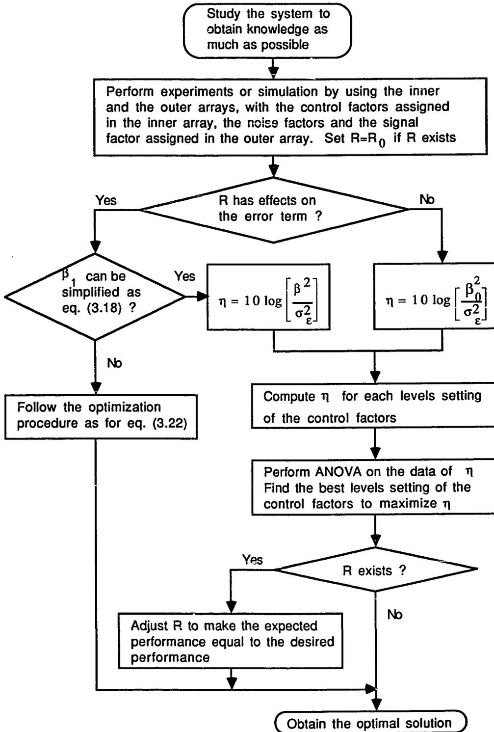
Figure 4.3. A flow chart for the optimization of dynamic systems
