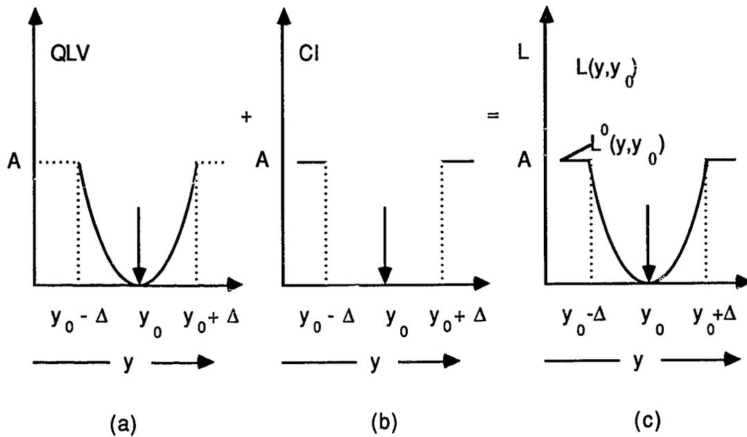
Figure 7.2. Best manufacturer's tolerance  $\Delta$ .
