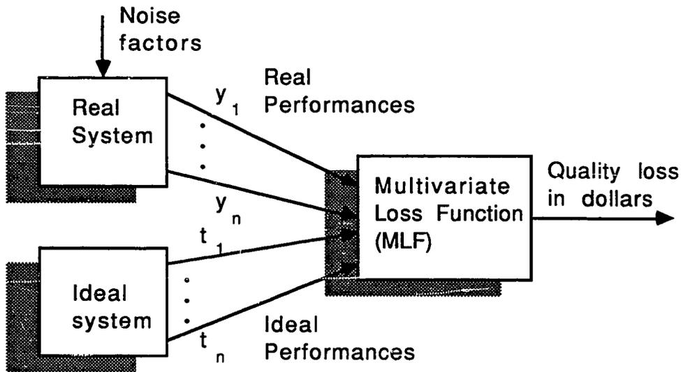
Figure 2.6. MLF transfers multivariate deviations to a loss in dollars
