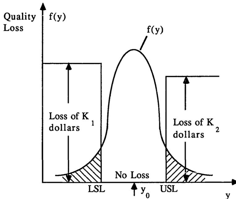
*Figure 2.2. Traditional quality evaluation (the shaded area is nonconforming portion)*
