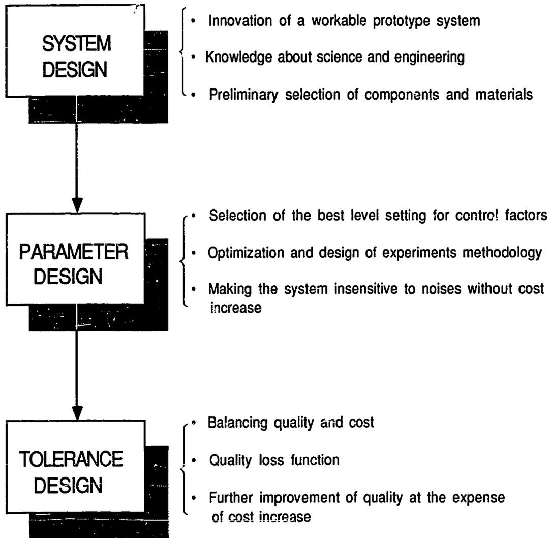
*Figure 1.1. Taguchi's robust design procedure.*
