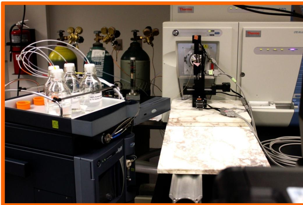
**Figure S5.3.** Picture showing the setup for LC-nSAII: Front view of Waters NanoAcquity liquid chromatography, Thermo LTQ-Velos mass spectrometer and, here, an automated x,y,z-stage for alignment of tip (**Figure 1a**) and the “picotip” extension (**Figure 1b**) of the fused silica capillary tube of the LC column placed about 0.1 mm out of the orifice inlet entrance of the mass spectrometer.
