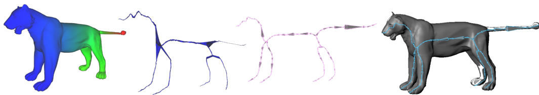
Figure 4.8: Automatic skeleton generation. From left to right: the first non-trivial eigenfunction of the loin model; shrink mesh based on iso-contours; skeleton generated with Reeb graph algorithm; and the embedding of the skeleton within the original model.
