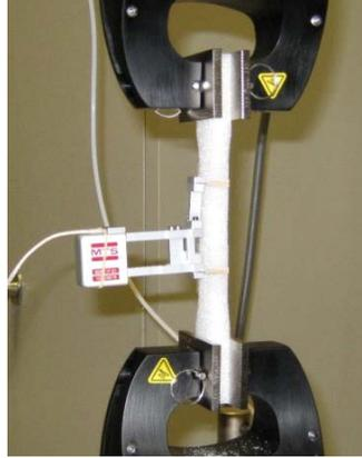
**Figure 4.12:** Typical test setup of the foam specimen showing the extensometer and clamp arrangements. Not readily visible are plastic protectors and double-sided tape used to prevent stress risers in the specimen.
