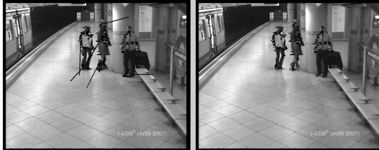
Figure 3.1: The KLT features before (left) and after (right) deleting the inaccurate features.
