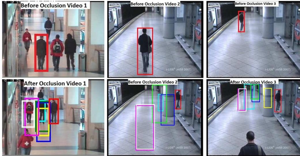
Figure 5.10: Recognizing targets after full occlusion. The systems are TLD (cyan), VTD (blue), MIL (green), JointSeg (yellow), LSH (magenta), DF (white) and our system (red).
