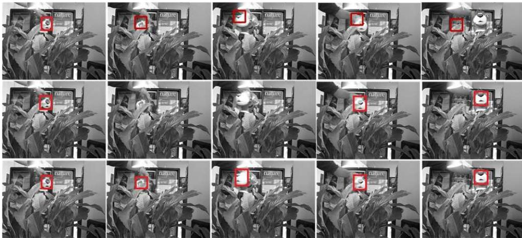
Figure 6.7: The tracking results of three different tracking systems: the appearance tracker (the first row), the appearance tracker with static CNN features (second row) and the appearance tracker with OCNN (the third row).
