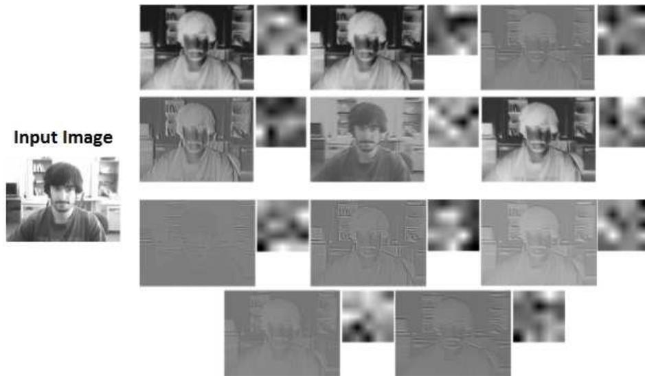
Figure 6.5: The results of running some convolutional layer kernels from the first and second layers on an image.
