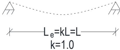
Figure 3: First buckled shape for simply supported member
