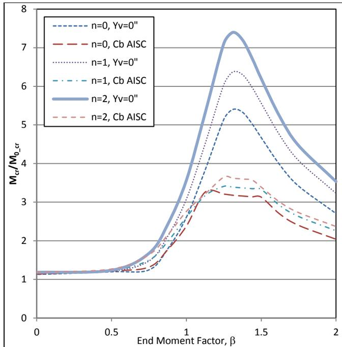
Figure 26: Load Type 3 code procedure comparison,  $n=0, 1$  and  $2$
