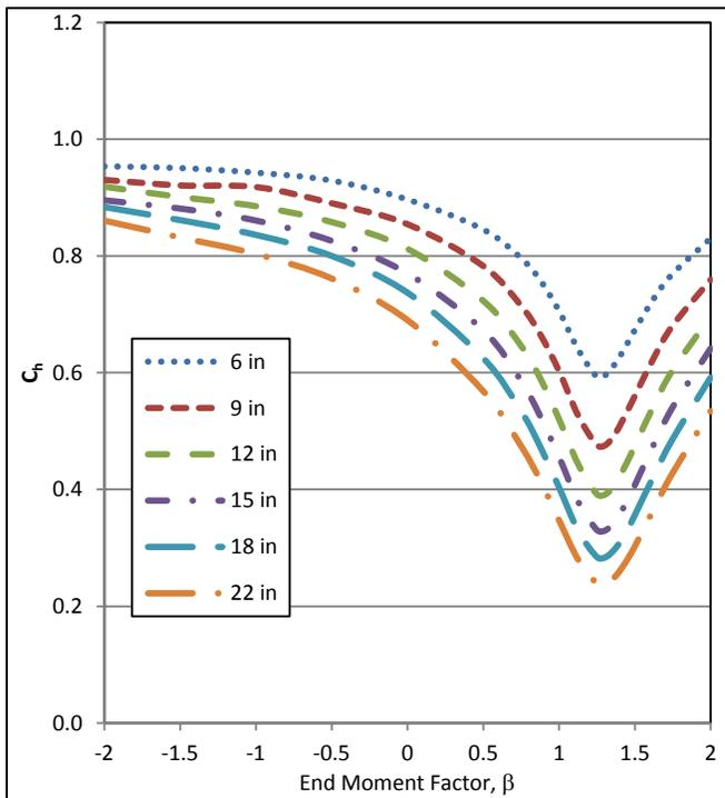
Figure 22: Load Type 3 load height factors,  $n=1$
