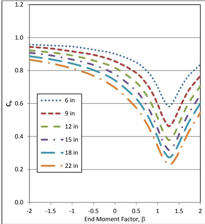
Figure 23: Load Type 3 load height factors,  $n=2$
