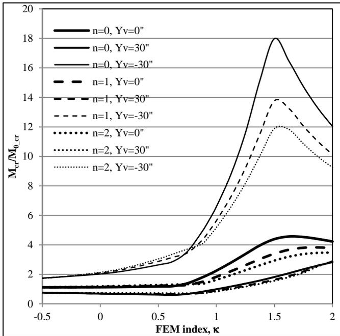
Figure 32: Load Type 2 load height effects,  $n=0, 1$  and  $2$
