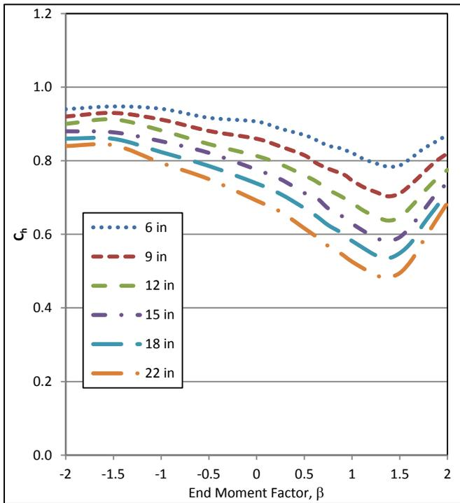
Figure 18: Load Type 2 load height factors,  $n=0$
