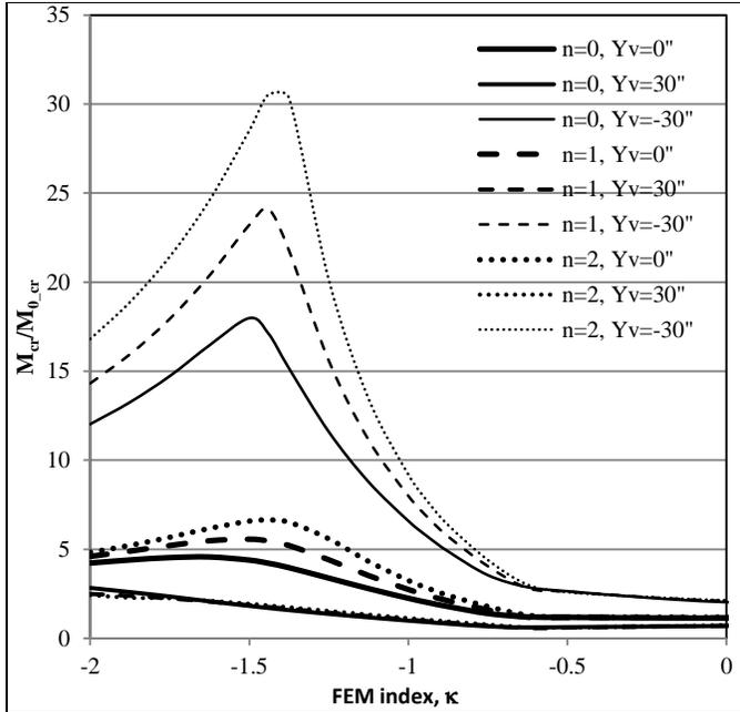
Figure 31: Load Type 1 load height effects,  $n=0, 1$  and  $2$
