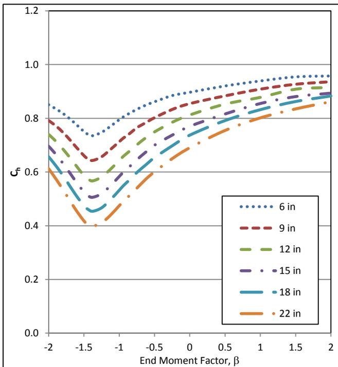
Figure 16: Load Type 1 load height factors,  $n=1$
