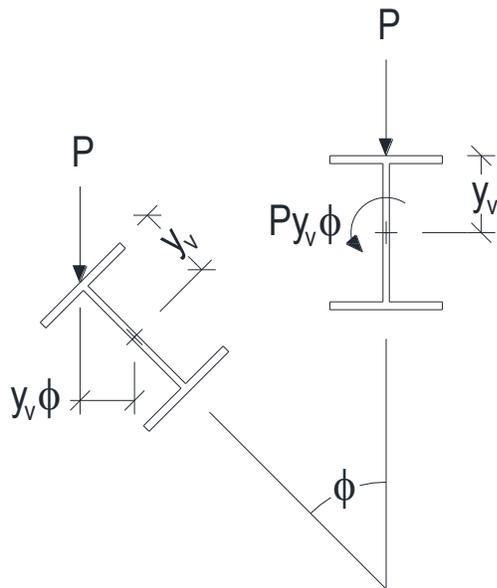
Figure 5: Free body diagram, load height analysis
