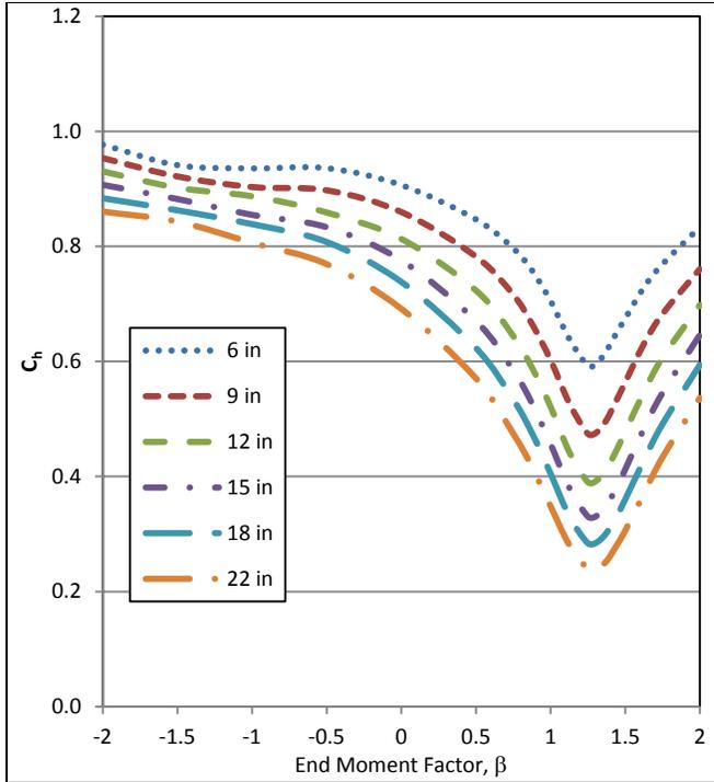
Figure 21: Load Type 3 load height factors,  $n=0$
