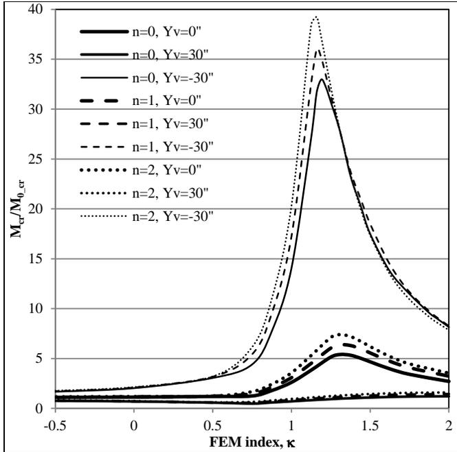
Figure 33: Load Type 3 load height effects,  $n=0, 1$  and  $2$
