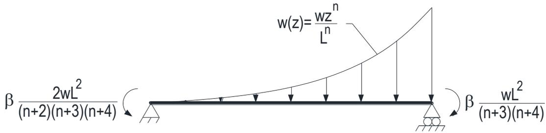
Figure 10: Spandrel load type with variable end moments
