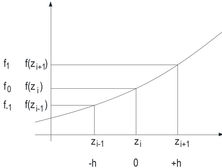
Figure 12: Central difference approximation for an arbitrary curve
