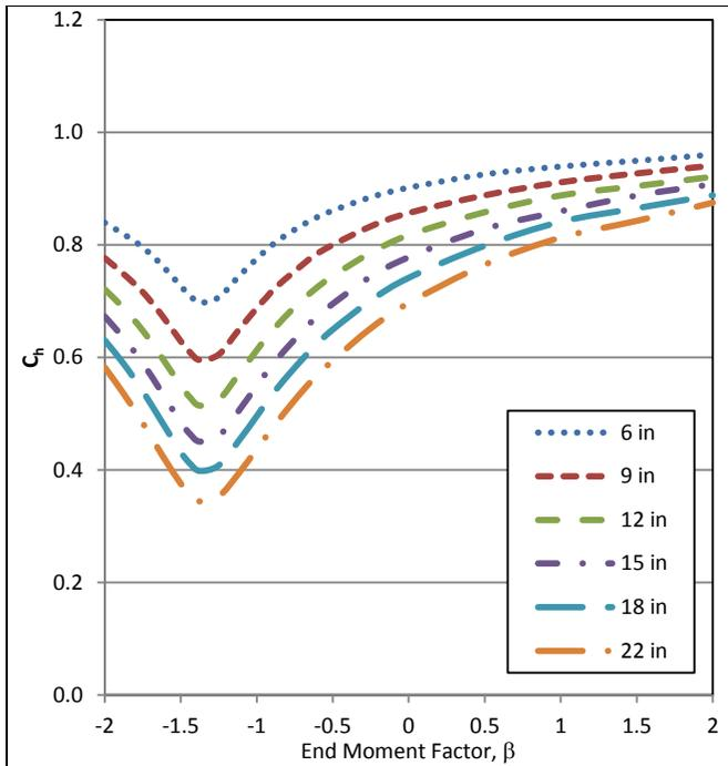
Figure 17: Load Type 1 load height factors,  $n=2$
