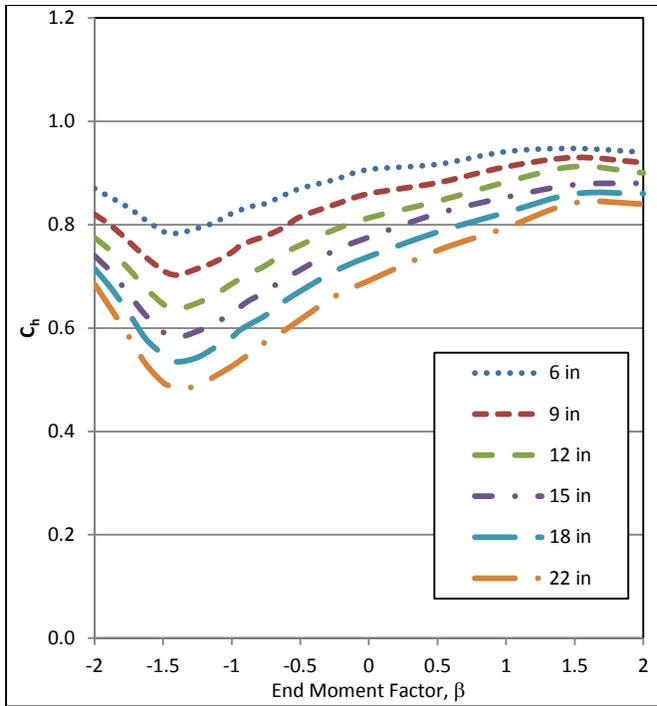
Figure 15: Load Type 1 load height factors,  $n=0$
