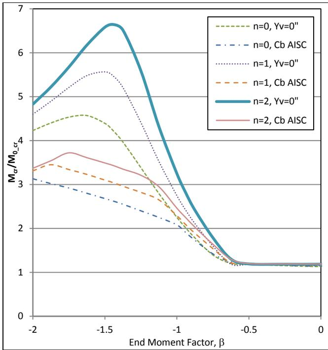
Figure 24: Load Type 1 code procedure comparison,  $n=0, 1$  and  $2$
