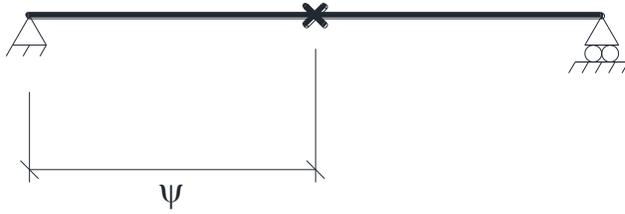
Figure 29: Discrete torsional brace
