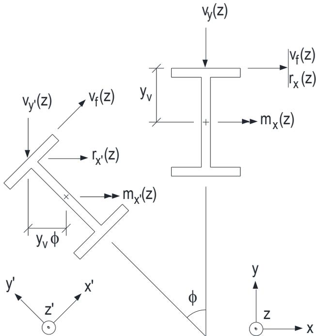
Figure 28: Restraint provided by continuous sources
