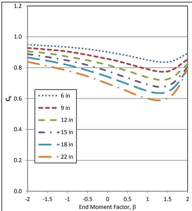
Figure 20: Load Type 2 load height factors,  $n=2$
