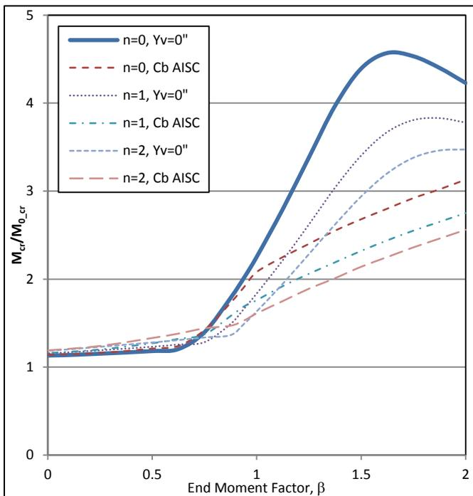
Figure 25: Load Type 2 code procedure comparison,  $n=0, 1$  and  $2$
