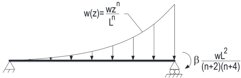
Figure 8: Spandrel load type with variable right end moment
