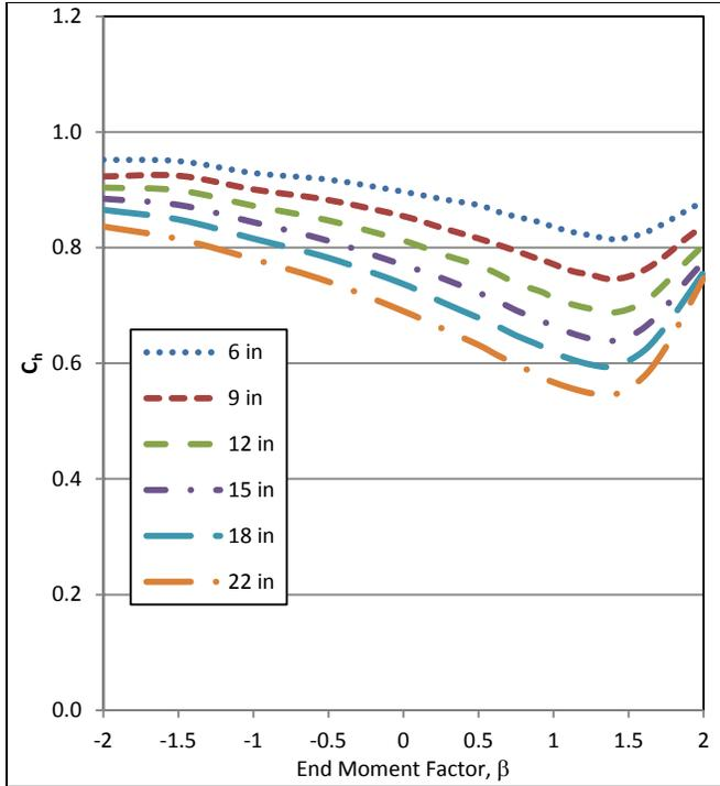
Figure 19: Load Type 2 load height factors,  $n=1$
