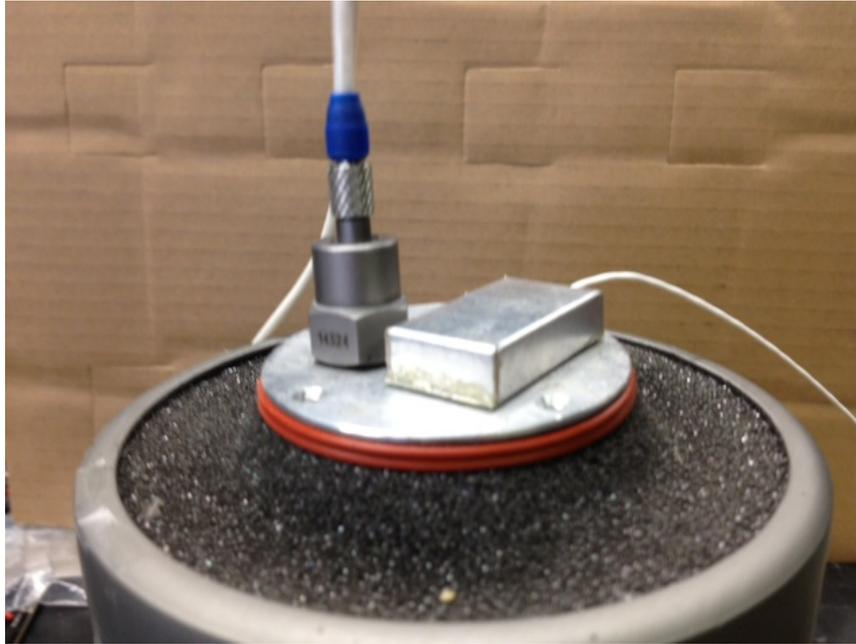
**Figure 3.2** The packaged device was mounted on a mechanical shaker. A commercial accelerometer was used to calibrate the acceleration.
