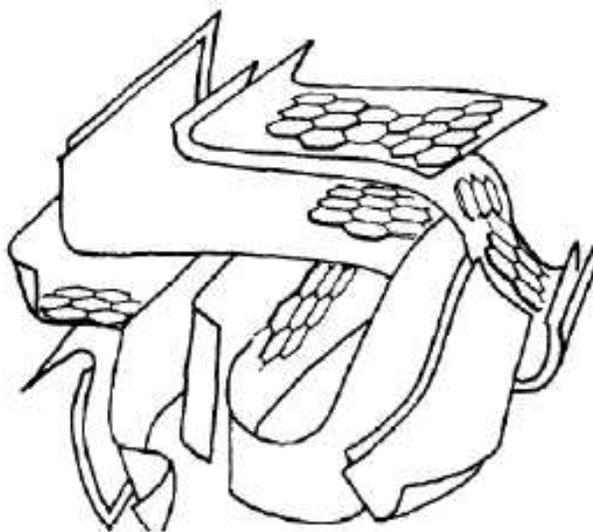
**Figure 11.** Structure of a typical microporous activated carbon.<sup>43</sup>
