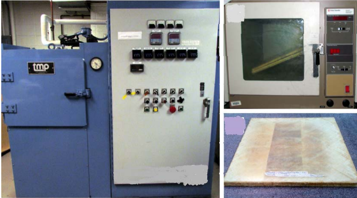
Fig. 3.3: Curing and post curing equipments.
