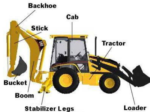
Figure 3: A typical backhoe and its parts (Photo courtesy of Caterpillar)
