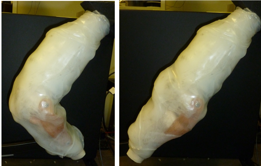
Figure 4.8: Knee Joint test stand with silicone ligaments and flesh; a) flexed, b) extended
