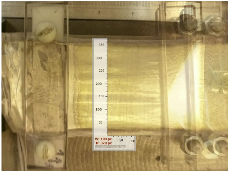
Figure 3.12: Pixel measurement of stretched ( \lambda=1.27 ) width of PolyPower DE film (stretched image is superimposed on image of unstretched material)
