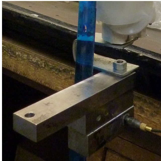
Figure 4.12: Weights used for oscillatory testing of knee joint (top = 0.28kg, middle = 0.18 kg, bottom = 0.177 kg)
