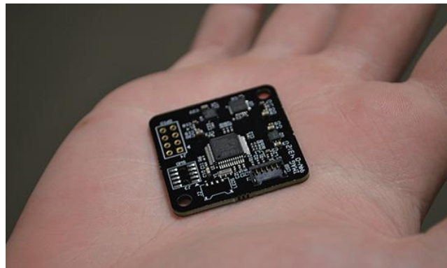
Figure 8. Oculus head tracking sensors [25]
