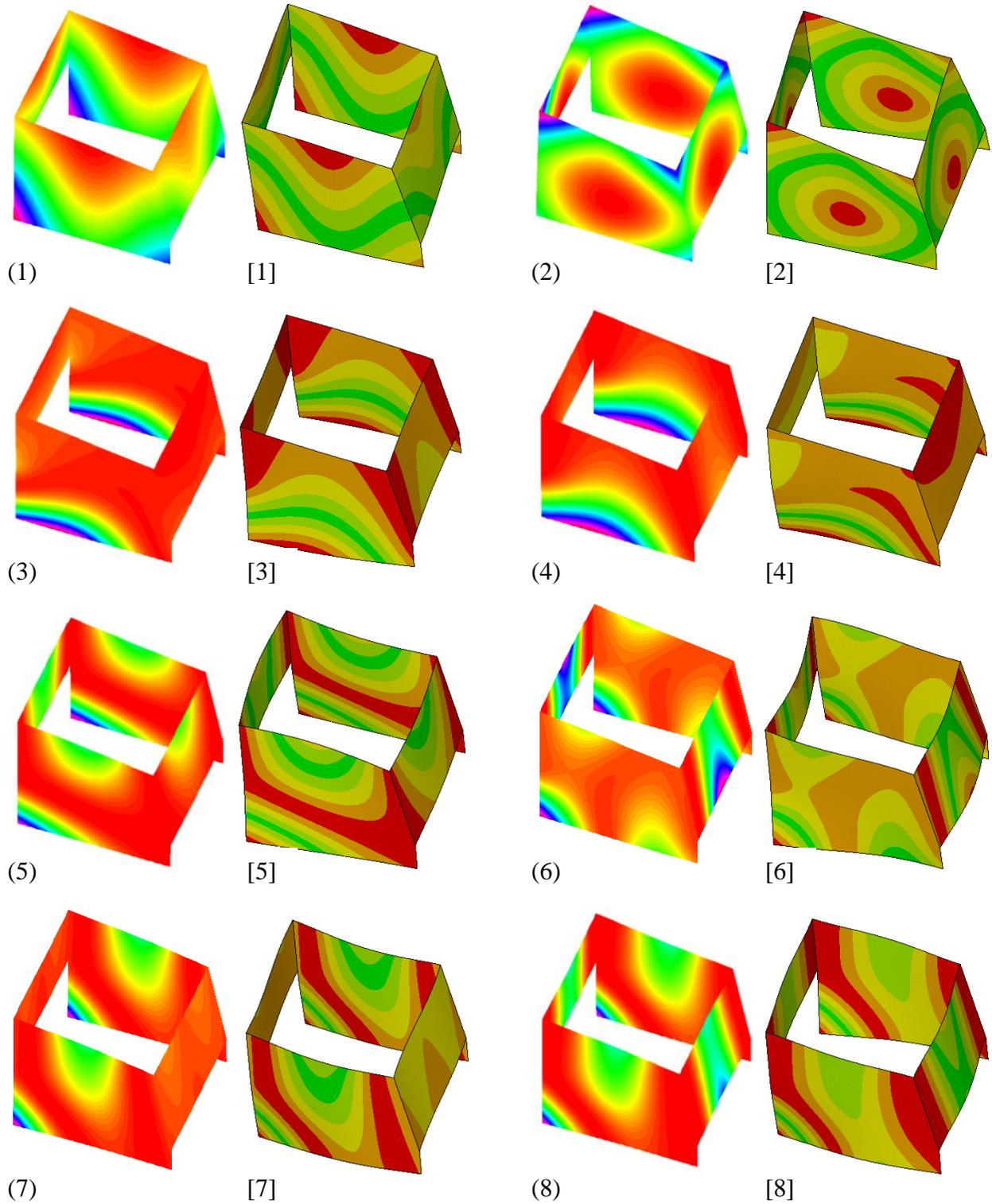
Figure 5.11 The first eight modes of the tested structure from current method (mode numbers in parentheses) and FEM method with 21,766 elements (mode numbers in brackets).
