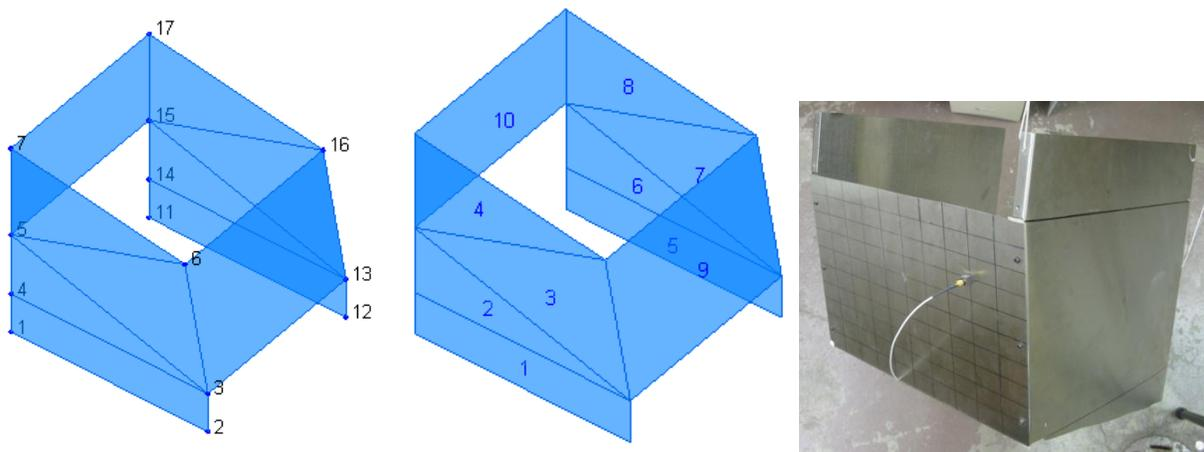
Figure 5.10 The evaluated general plate structure with a) corner numbers at the plate corners, b) plate numbers at the plate centers, and c) lab setup.
