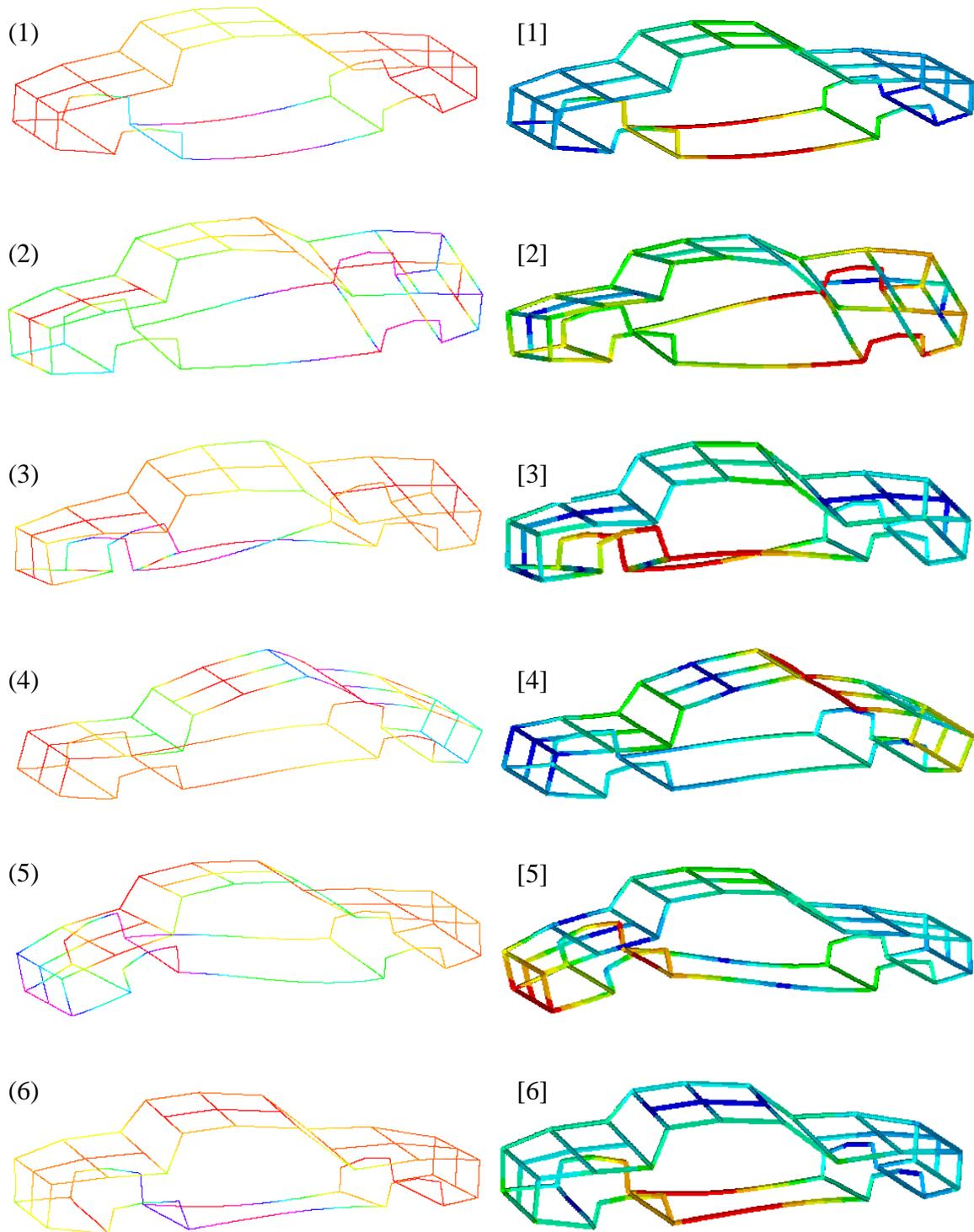
Figure 5.13 The first six mode shapes of the car frame from current method ( left side and indexed in parenthesis) and FEM method with 2173 elements (right side and indexed in square brackets)
