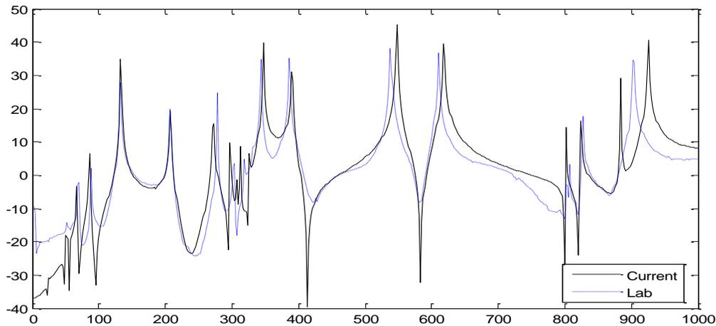
Figure 5.8 FRF curves of the 3-D frame with input force at 0.25L of beam 4 in z direction and response measured at 0.3L of beam 1 in y direction.
