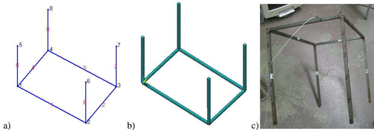
Figure 5.4 A rigidly connected 3-D frame. a) Setup used in current method with corner numbers at the frame corners and beam numbers in the middle of the beams. b) FEM model c) Lab setup with the same number sequence as current and FEM models.
