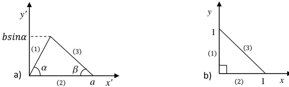
Figure 4.2. A triangular plate before (a) and after (b) coordinator transformation
