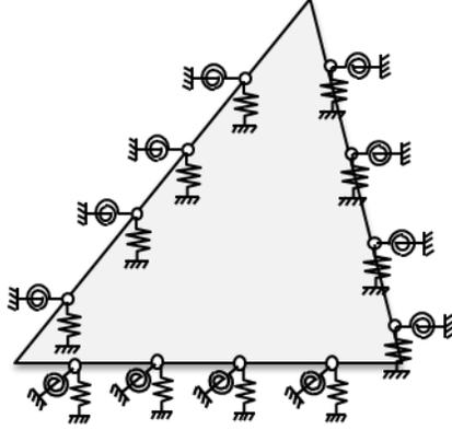
Figure 4.1. A general triangular plate with elastically restrained edges.
