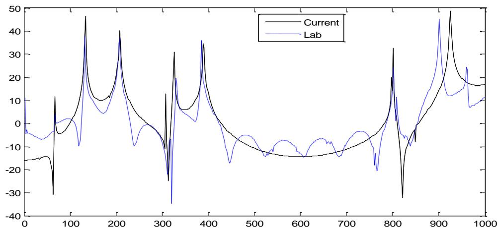
Figure 5.7 FRF curves of the 3-D frame with input force at  $0.5L$  of beam 1 in  $y$  direction and response measured at  $0.3L$  of beam 5 in  $y$  direction.
