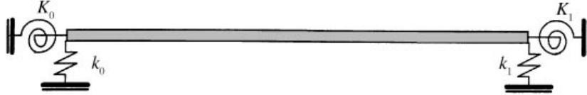
Figure 2.1 A beam elastically restrained at both ends
