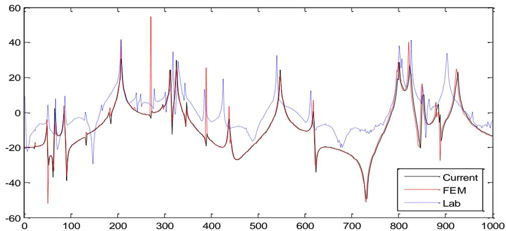
Figure 5.6 FRF curves of the 3-D frame with input force at  $0.6L$  of beam 3 in  $y$  direction and response measured at  $0.3L$  of beam 7 in  $y$  direction.
