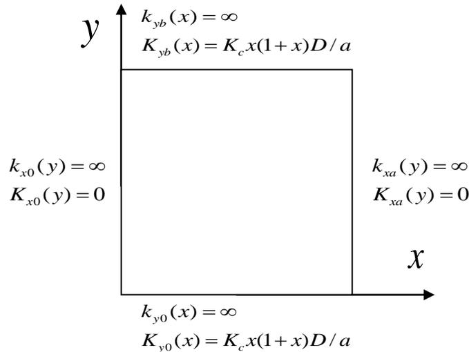
Figure 3.3 A simply supported plate with rotational springs of parabolically varying stiffness along two opposite edges, where  $K_c$  is a constant.
