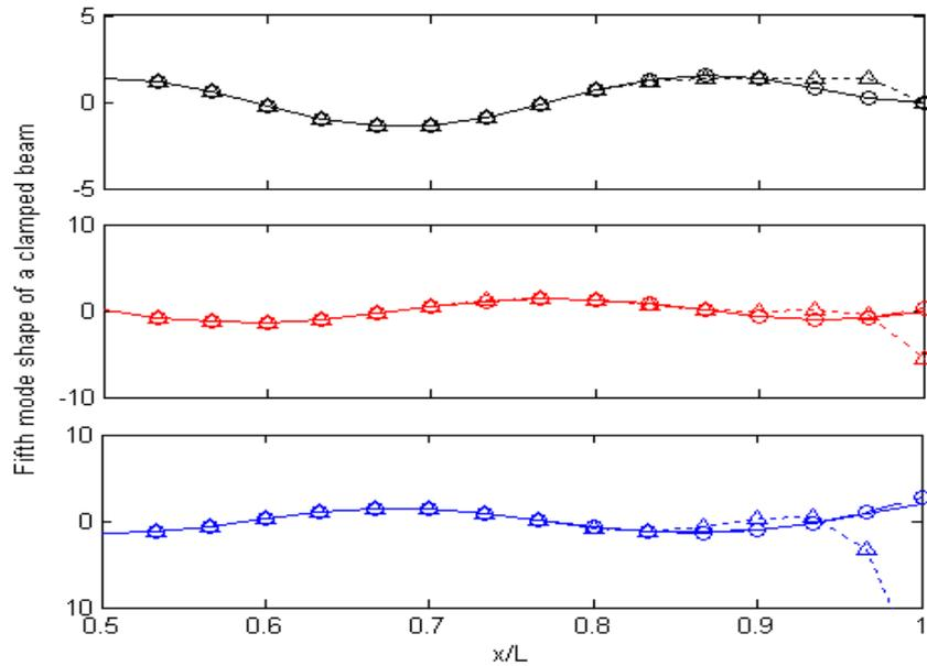
Figure 1.1 A comparison of the DQ interpolation scheme and current FSEM method: Original beam function (black), the first derivative (red), the second derivative (blue); DQ with traditional Legendre interpolation function (triangle); Current method (circle)
