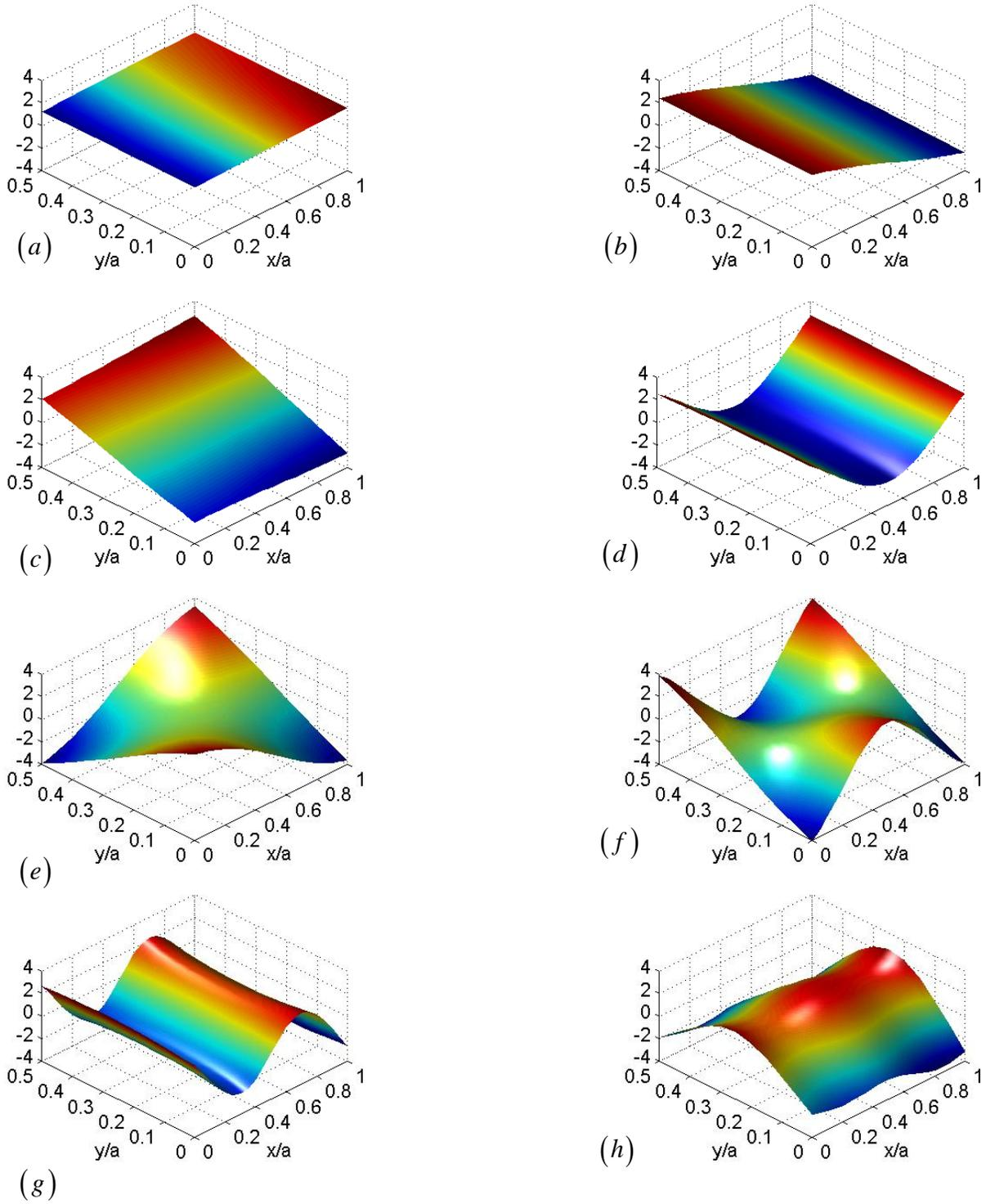
Figure 3.5. The (a) first, (b) second, (c) third, (d) fourth, (e) fifth, (f) sixth, (g) seventh and (h) eighth mode shapes for a plate with aspect ratio  $r = 2$  and boundary condition described in Figure 3.4.
