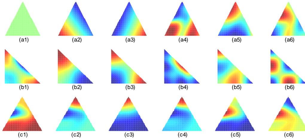
Figure 4.3. The first six mode shapes of a free equilateral triangular plate as described in Section 4.6.1 (a1-a6), a right-angled isosceles triangular plate with elastic boundary constraints  $k = 10$  and  $K = 100$  as described in Section 4.6.3 (b1-b6), and an anisotropic plate with  $\beta = 30^\circ$  and elastic boundary constraints  $k = 100$  and  $K = 50$  as described in Section 4.6.4 (c1-c6).
