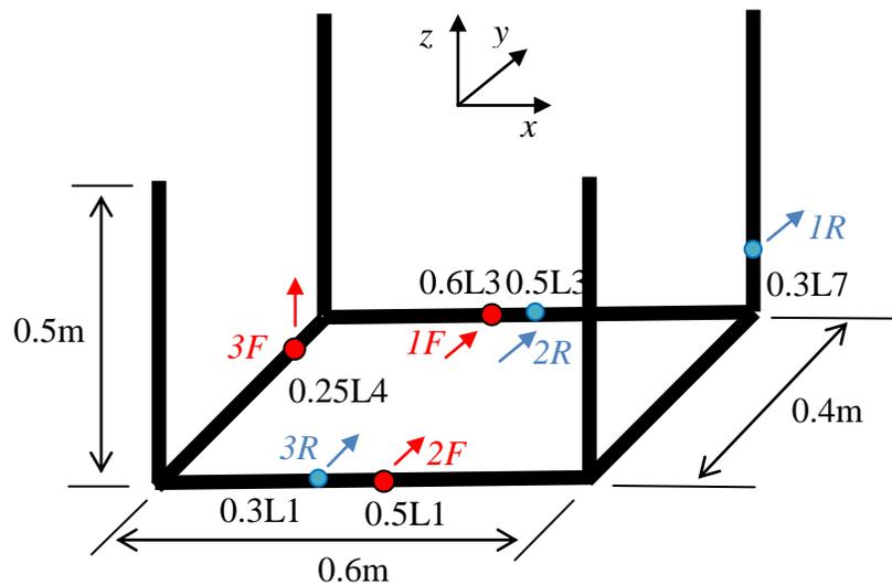
Figure 5.5 A scheme showing the input force and response locations.
