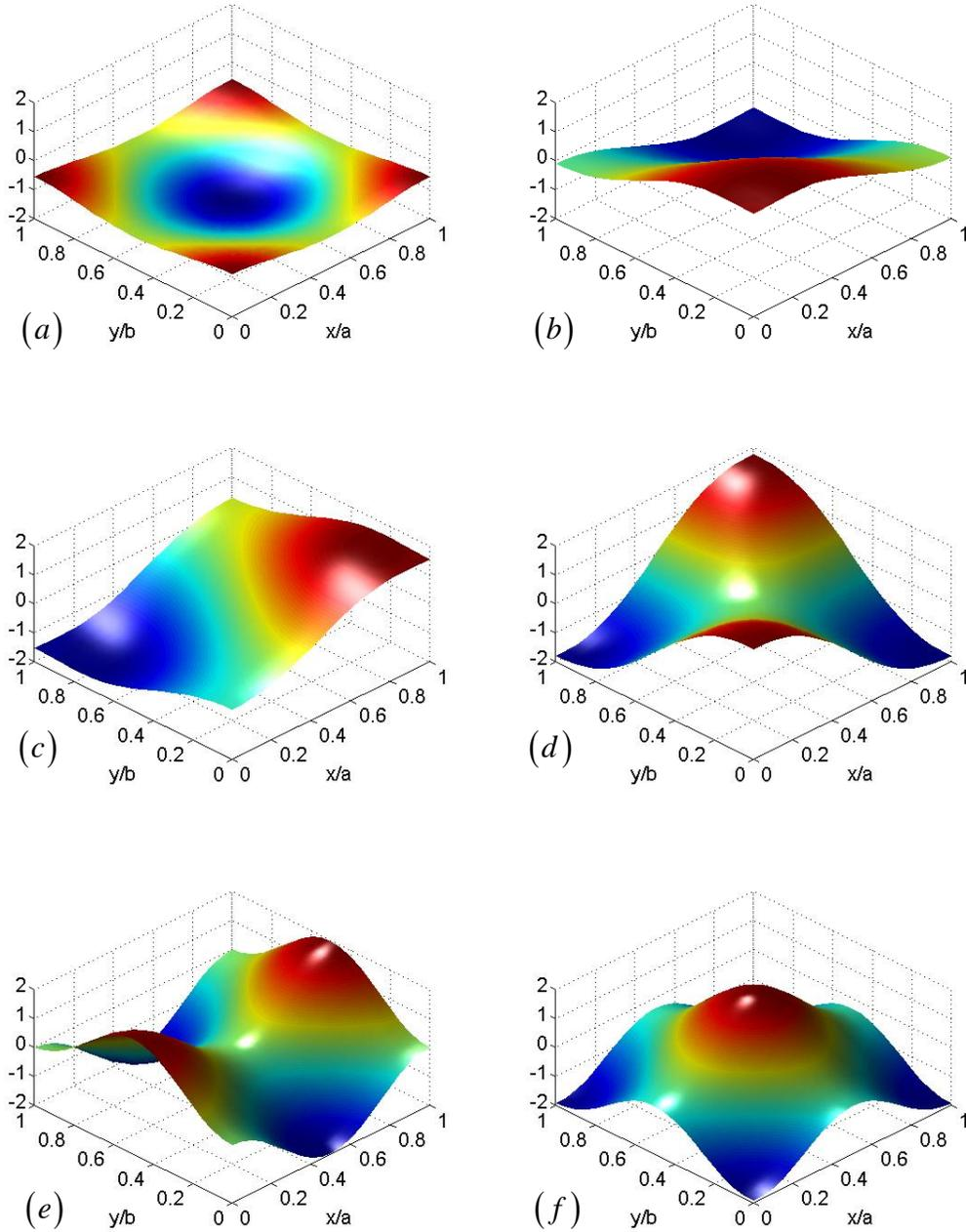
Figure 3.2. The (a) first, (b) second, (c) third, (d) fourth, (e) fifth, and (f) sixth mode shapes of a square plate with  $ka^3/D = 100$  and  $Ka/D = 1000$  at all four edges.
