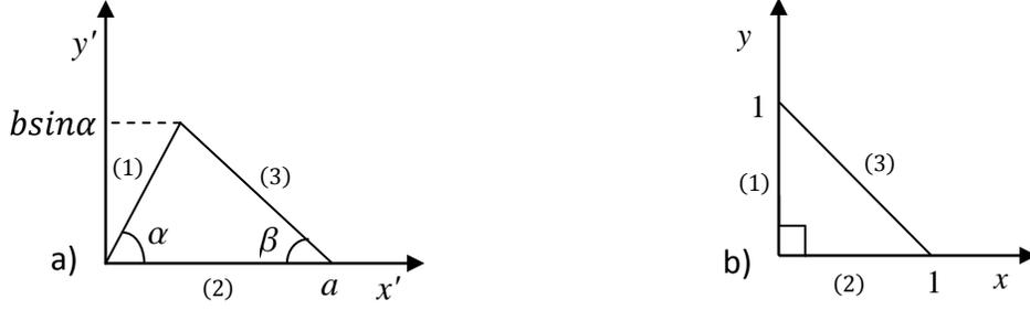
Figure 5.3 A triangular plate before (a) and after (b) coordinate transformation
