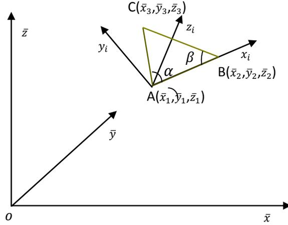
Figure 5.2 Transformation between the local and global coordinates
