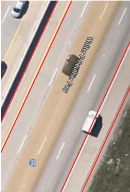
(a) User cannot set widths for the road individually when the size of shoulders are different
