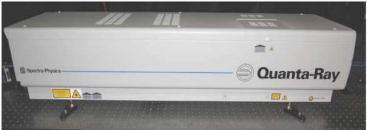
Figure 3.2 The high-energy Lab 150-10 nanosecond laser system used in this research from Spectra-Physics.
