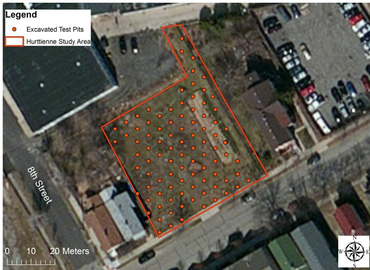
Figure 24. Excavated test pits at Hurttienne lot.
