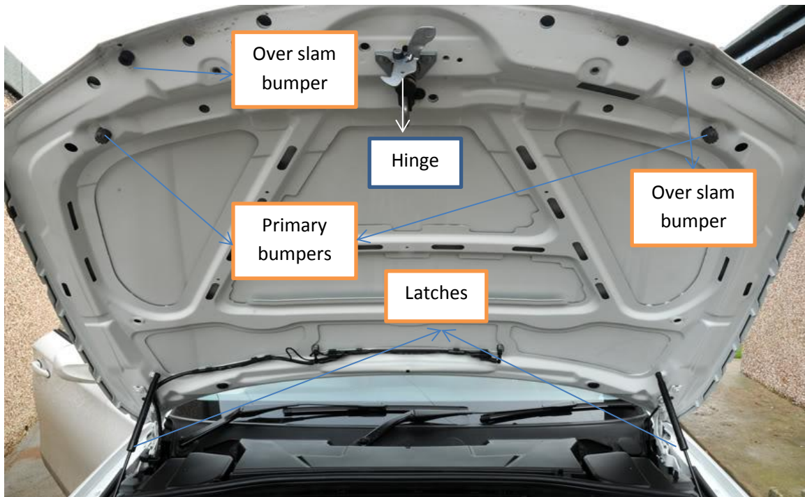
Figure 24: Geometry of a typical hood (Honda Accord, 2014)
