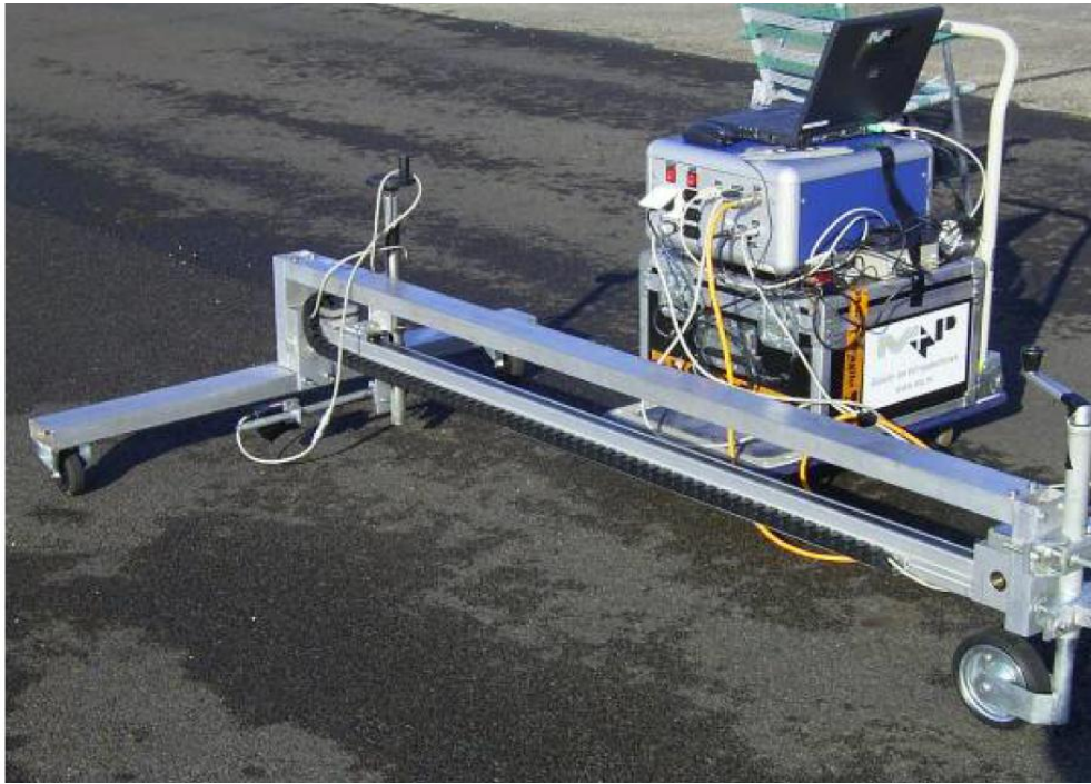
Figure 7: M+P static (3D) road surface roughness measurement system [8]
