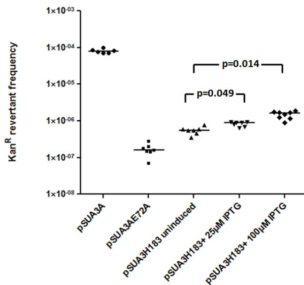
**Figure 15:** Kanamycin resistance reversion assay results for pSUA3H183. The median value is shown by the horizontal bar.
