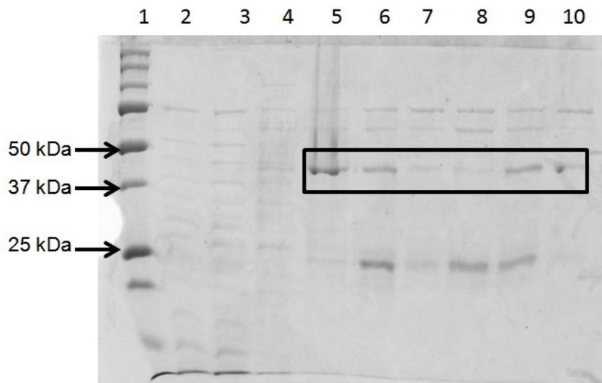
**Figure 12:** 12% SDS-PAGE gel for GSTA3H200 purification.
