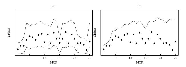
Figure 13: Hypothesis test results comparison between the proposed PH model (a) and Wu & Meeker (2002) (b) for warranty claims from vehicles during the fourth month in service.
