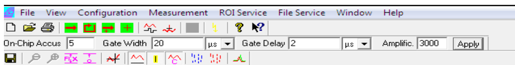
Figure 3.18: The control menu of the ESAWIN software which controlled the timing of the laser and spectrometer.
